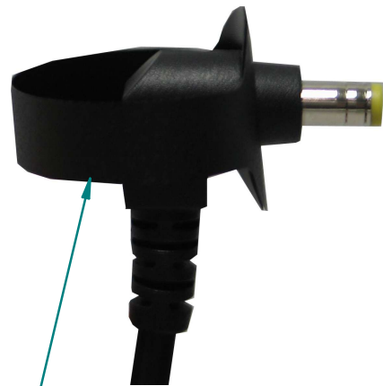
Figure 5 Power Cable Pull Strap
