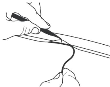
2. Route the cable from the antenna to the vehicle's interior by tucking it underneath the rubber molding around rear window, as shown below.
