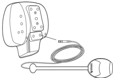
2. Find an antenna location on a metal surface of your vehicle at least 12" x 12", and at least 6" from a window.
