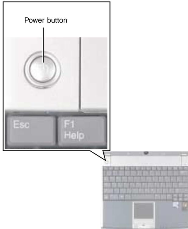
The power button is preset to On/Off mode. However, you can also set it to function in Standby/Resume mode. For instructions on changing the power button mode, see “Changing power settings” on page 155.
