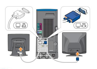
**Connect one monitor**If your monitor has a DVI connector, plug it into the DVI connector on the computer. If your monitor has a VGA connector, plug it into the VGA connector on the computer.
