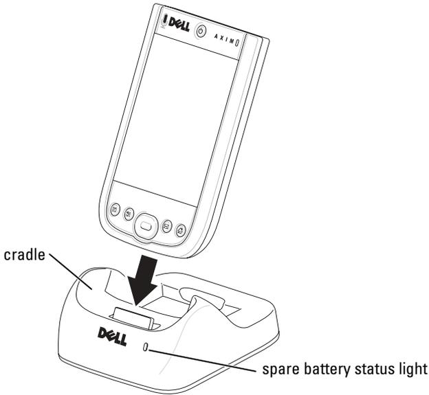
When the device is docked in the cradle, the power button on the device turns on and the connection status icon appears on the command bar (see page 65).
