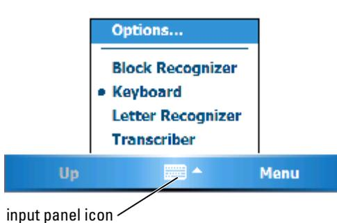
To show or hide the input panel, tap the input panel icon. Tap the arrow next to the input panel icon to change the input method.
