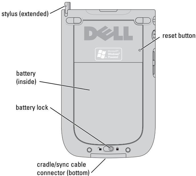
**BATTERY LOCK** — Use this switch to release and remove the main battery. See "Installing and Removing the Battery" on page 48.
