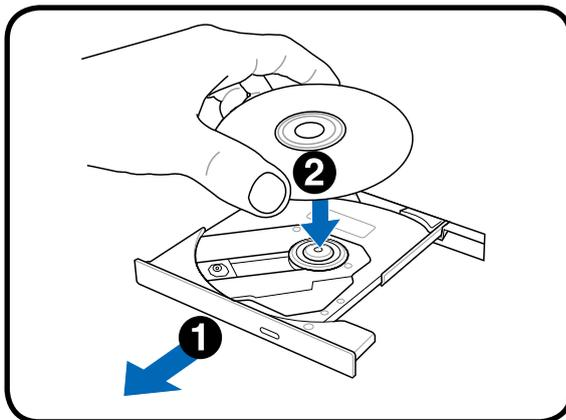
3. Hold the disc by the edge and face the disc's printed side up. Push down on both sides of the disc's center until the disc snaps onto the hub. **The hub should be higher than the disc when correctly mounted.**
