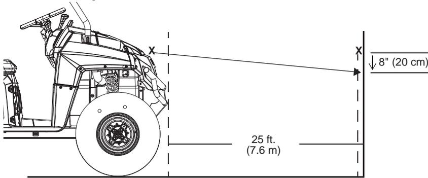
1. Place the vehicle on a level surface with the headlight approximately 25 ft. (7.6 m) from a wall.
