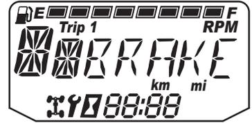
**Tip:** This feature will not operate properly if the park brake connector or switch (under the hood) malfunctions or becomes disconnected, or if the switch has moved. Check for disconnection, then see your dealer promptly if this feature fails to operate properly.
