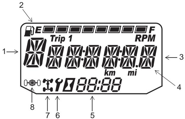
1. **Gear Indicator** - This indicator displays gear shifter position.
