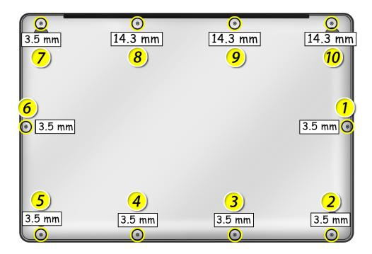
5 Tilt up and remove bottom case.
