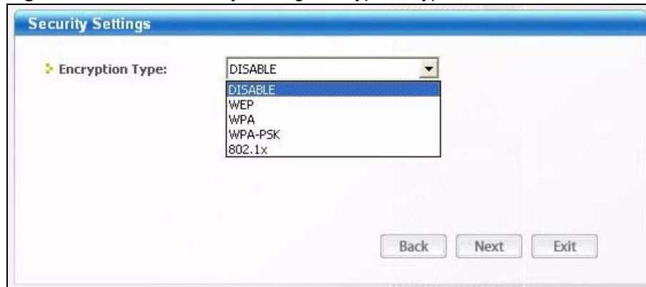
Figure 31 Profile: Security Setting: Encryption Type
