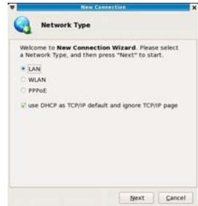
1. On the above menu, click the mouse to tick “LAN” and click the front panel of the item “use DHCP as TCP/IP default and ignore TCP/IP page” to cancel the tick, then click “Next” to enter the window of “TCP/IP Settings” as shown right:
