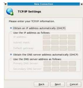
On the menu, you need to input the IP addresses, subnet masks, default gateway, DNS and etc, then click “Next” to enter the window of “Summary” to tick the item “Connect after finish”, then the system will start connecting the network. After several seconds, click the icon
