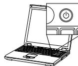
The DC push-button on/off switch on the system does not turn off system AC power. To remove AC power from the system, you must unplug each AC power cord from the wall outlet or power supply.
