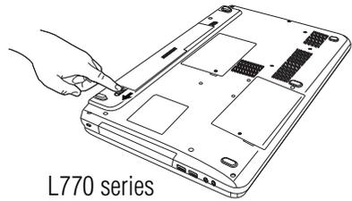
*(Sample Illustration) Unlocking the battery release lock*
