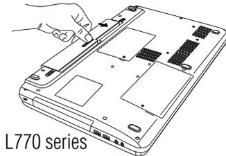
*(Sample Illustration) Inserting the battery*
