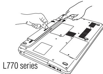
*(Sample Illustration) Removing the battery*
