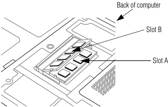
*(Sample Illustration) Removing the memory module*
