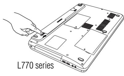
*(Sample Illustration) Locking the battery release lock*
