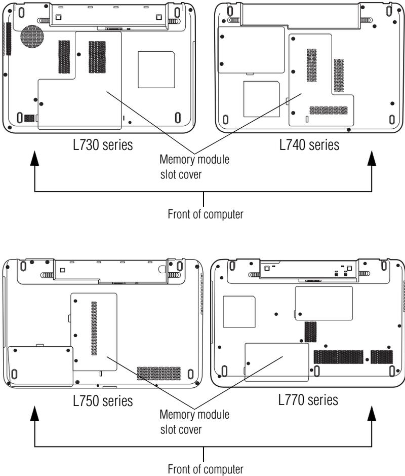
*(Sample Illustration) Locating the memory module slot cover*
