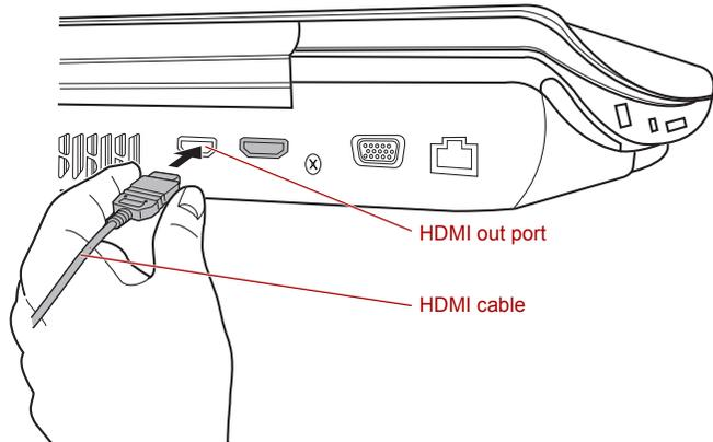
Figure 8-11 Connecting the HDMI out port
