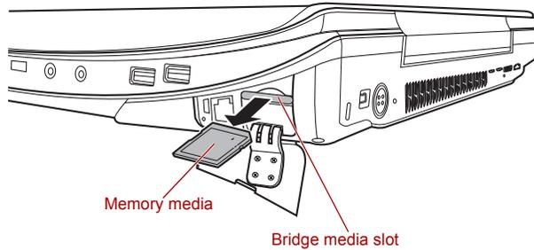
Figure 8-5 Removing memory media
