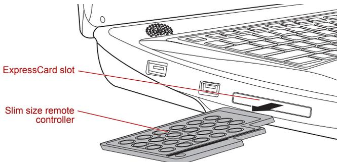
Figure 4-16 Removing a Slim size remote controller
