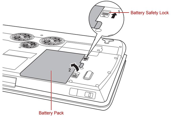
*Figure 6-2 Releasing the battery pack (2)*
