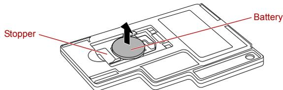
*Figure 4-14 Removing the batteries*
