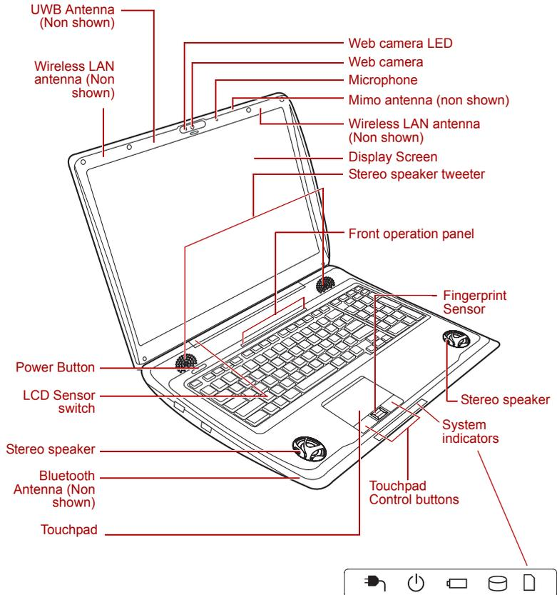
Figure 2-6 The front of the Touch Pad model with the display open
