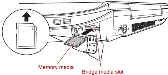
*Figure 8-4 Inserting a memory media*
