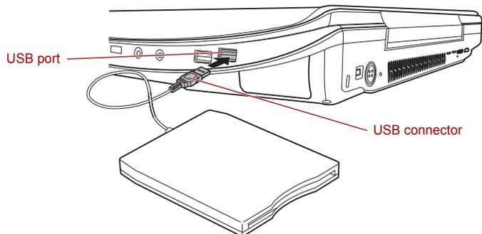
Figure 8-8 Connecting the USB floppy diskette drive
