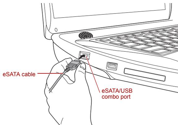
*Figure 8-9 Connecting an eSATA cable to the USB (eSATA combo) port*
