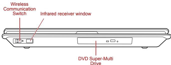
*Figure 2-1 Front of the computer with display closed*
