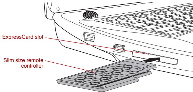
Figure 4-15 Inserting a Slim size remote controller
