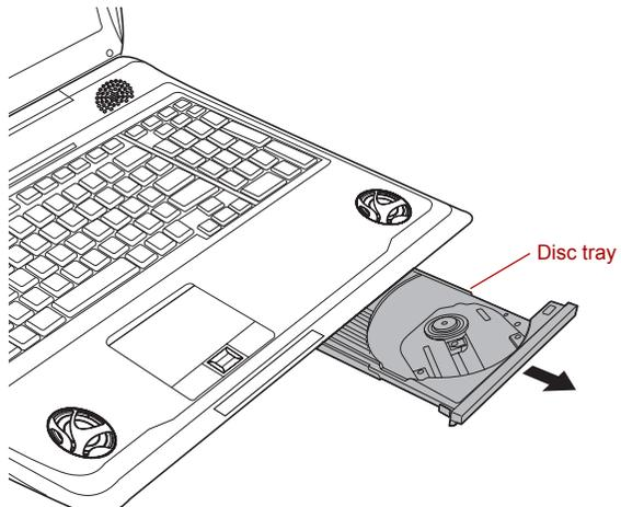
*Figure 4-5 Pulling the disc tray open*
