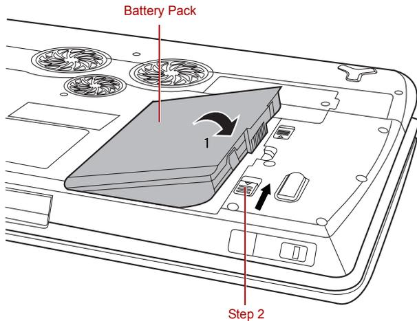
*Figure 6-3 Securing the battery pack*
