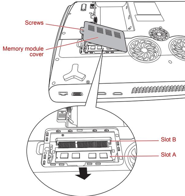
*Figure 8-6 Removing the memory module cover*
