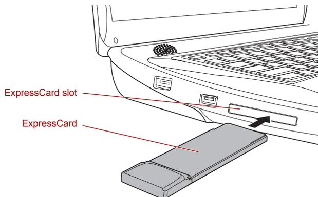
*Figure 8-1 Inserting the ExpressCard*
