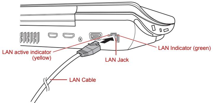
Figure 4-18 Connecting the LAN cable
