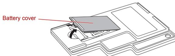
Figure 4-11 Opening the battery cover
