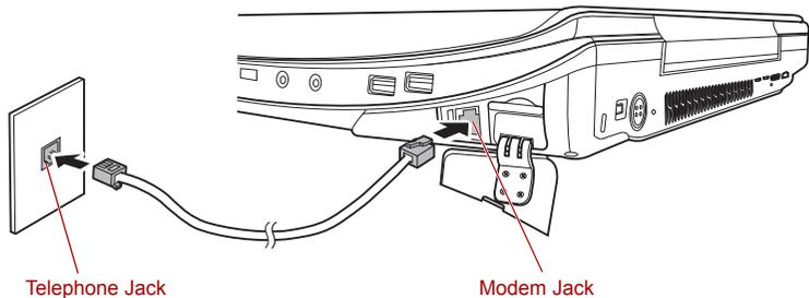
*Figure 4-17 Connecting the internal modem*
