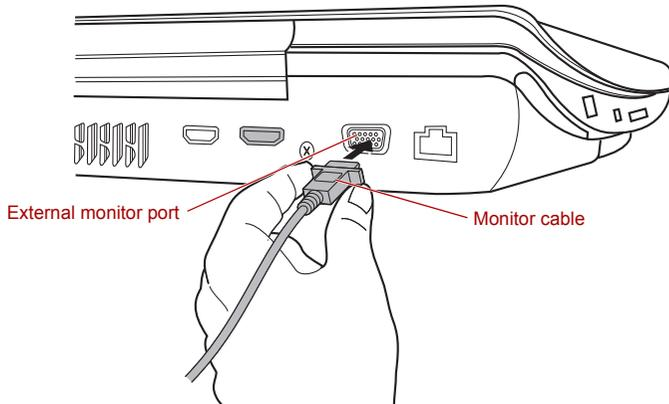
Figure 8-10 Connecting the monitor cable to the external monitor port
