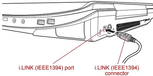
*Figure 8-12 Connecting the i.LINK (IEEE1394) port*
