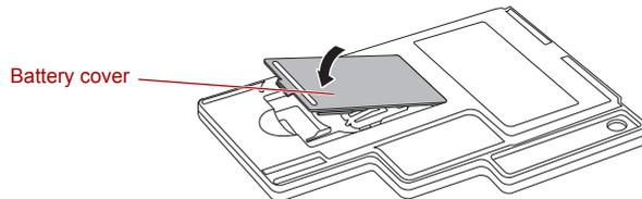
*Figure 4-13 Closing the battery cover*
