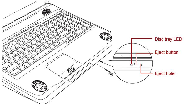
Figure 4-8 Manual release with the eject hole
