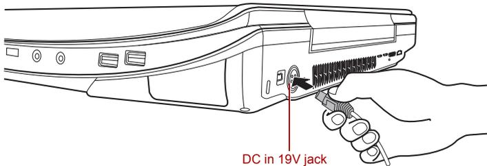
*Figure 3-2 Connecting the adaptor to the computer*
