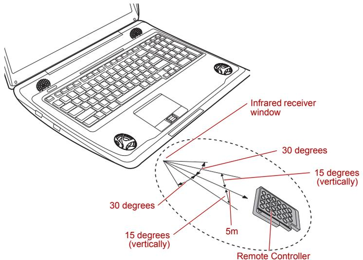
*Figure 4-10 Operational range of the remote control*
