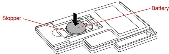
*Figure 4-12 Inserting the battery*
