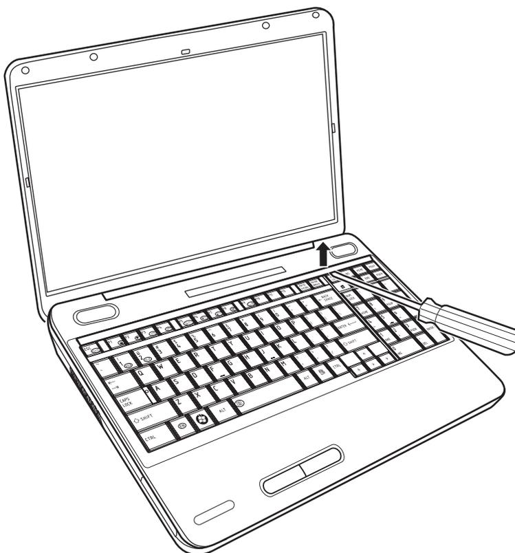
*Figure 4.8 Removing the keyboard cover*
