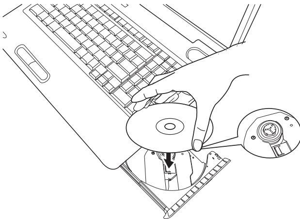
Figure 4-4 Inserting a CD/DVD/BD
