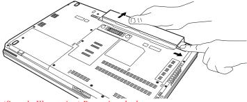
(Sample Illustration) Removing the battery
