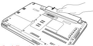
(Sample Illustration) Inserting the battery
