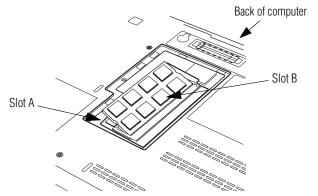
(Sample Illustration) Removing the memory module
