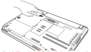
(Sample Illustration) Unlocking the battery release lock
