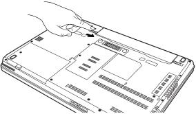
(Sample Illustration) Locking the battery release lock
