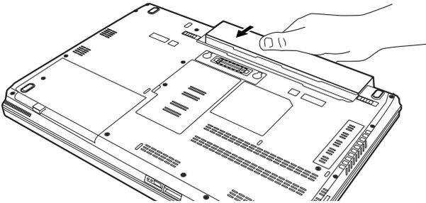
*(Sample Illustration) Inserting the battery*
