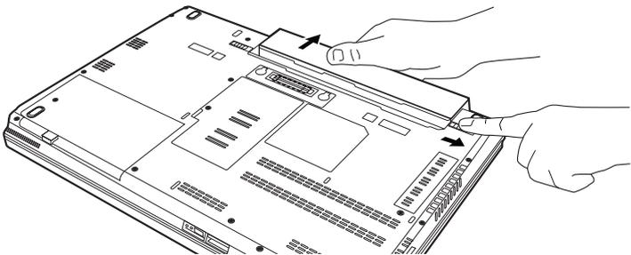
*(Sample Illustration) Removing the battery*
