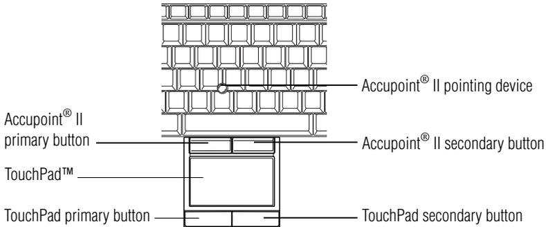
*(Sample Illustration) Toshiba Dual Pointing Device buttons*
