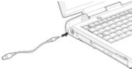
Figure 8-14 Connecting a television
