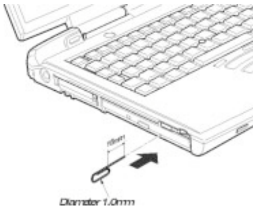
Figure 4-6 Manual release with the eject hole
