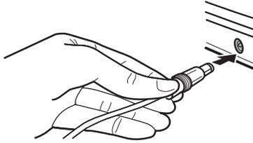
*(Sample Illustration) Connecting the AC adaptor cord to the computer*
