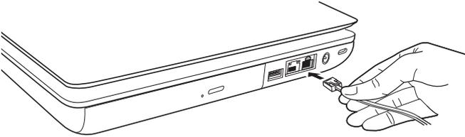
*(Sample Illustration) Connecting the telephone cable to the modem port*
