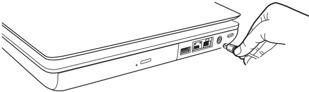
*(Sample Illustration) Connecting the AC adaptor cord to the computer*
