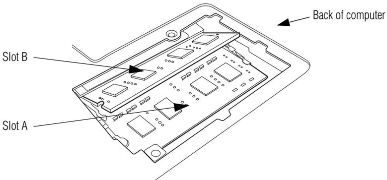
*(Sample Illustration) Removing the memory module*
