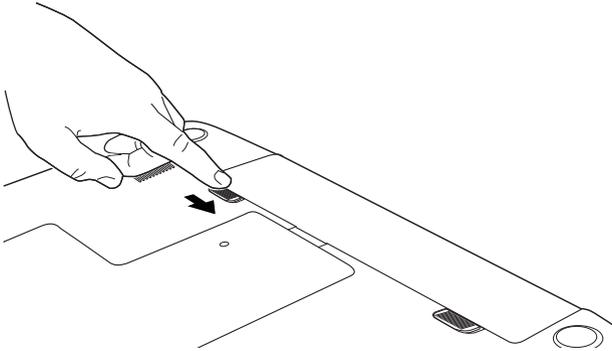
*(Sample Illustration) Locking the battery release lock*
