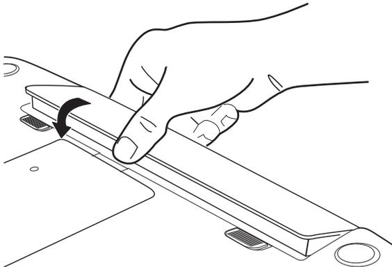
*(Sample Illustration) Inserting the battery*
