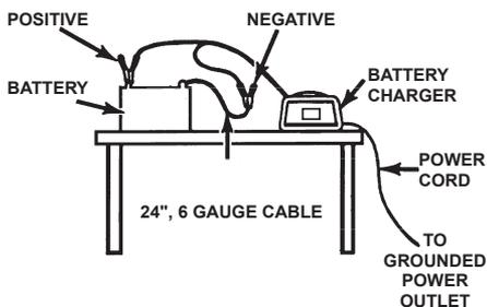
1. Note the polarity of the battery posts by checking the identification marks on the battery: POSITIVE (POS, P or +) and NEGATIVE (NEG, N or -). The positive post is usually larger than the negative post.
