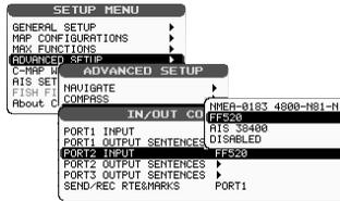
Figure 2.4.0 - Selecting the FF520 on CP180/CP180i/CPV350
