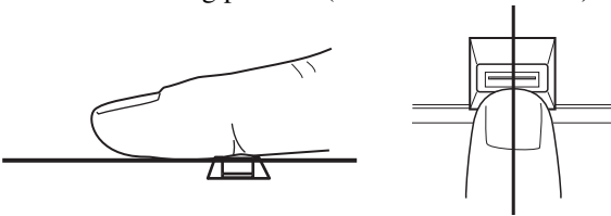
(Sample Illustration) Aligning the finger on the reader
