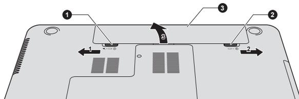
Figure 5-2 Releasing the battery pack -2
