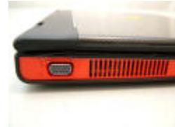
On the right, we find a standard DB-15F External VGA display port for monitors and projectors next to the ventilation slots.
