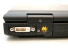
A DVI-D and S-video/TV-out (NTSC/PAL) port lets you connect the Acer Ferrari 4000 to a wide range of supported devices.
