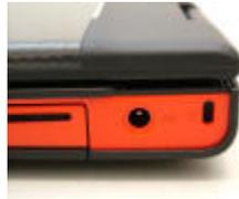
On the left side of the laptop, is the Acer Power Jack, and a security key lock that accepts any Kensington-compatible Computer Security Lock.
