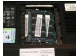
The *Acer Ferrari 4000* comes with 1GB of DDR333 RAM. It can be expanded to 2GB; but with only 2 sockets available for memory, you'll have to remove these two 512MB soDIMMs first.
