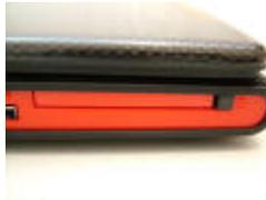
Up front is the Type II PC Card slot with removable dust cover, and the PC Card slot eject button.
