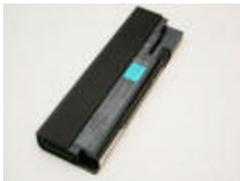
The 71 W Li-ion battery fully charges in 2.5 hours, and lasts for 3.5 hours in use—not bad for a laptop with this much power.
