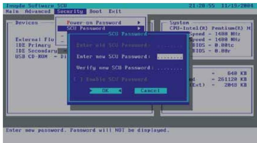
Allows you to set the password for entering SCU Setup. When typing the password, first make sure that Num Lk is off, and then type the password in the entry fields and press Enter. Confirm your password by typing it again and pressing Enter. If the **Enable SCU Password** sub-item is enabled, the SCU password is always required to enter SCU Setup.
