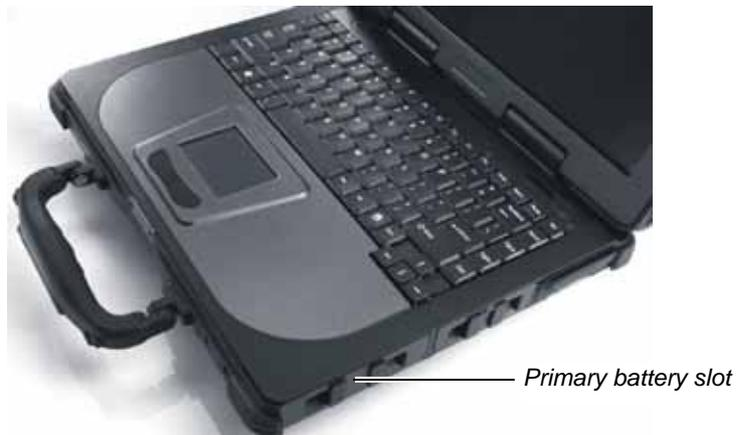
2. Open the slot cover by pressing on both sides of the release latch using your thumb and index fingers.
