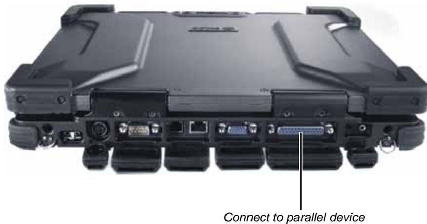
4. If the parallel device has independent power, plug its power cord into an electrical outlet.
