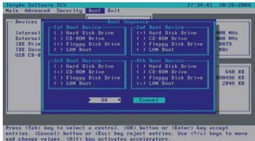
Sets the first, second, third, and fourth booting device. The system will try to boot from the first device but if it is not available, will try the next boot device. If you set the first boot device to *LAN Boot*, the system will boot from the LAN server first. The options are *Hard Disk Drive*, *CD-ROM Drive*, *Floppy Disk Drive*, and *LAN Boot*.
