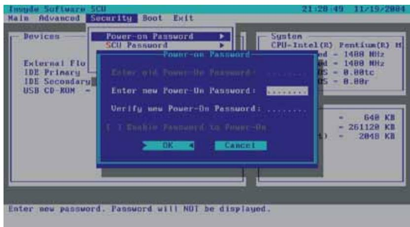
Allows you to set the password for booting-up your system. When typing the password, first make sure that Num Lk is off, and then type the password in the entry fields and press Enter. Confirm your password by typing it again and pressing Enter. If the **Enable Password to Power-on** sub-item is enabled, the power-on password is always required to boot the computer.
