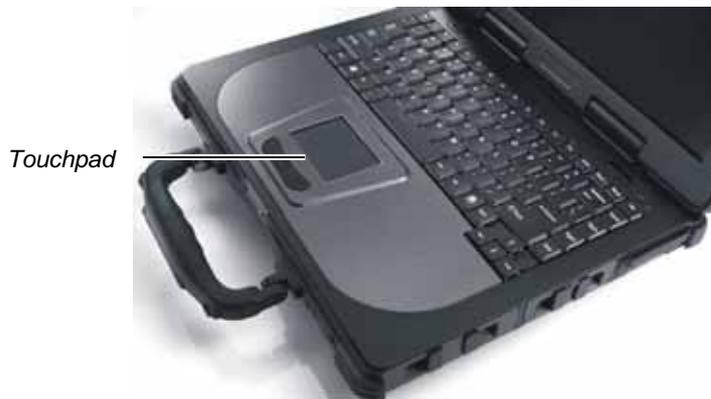
The touchpad consists of a rectangular pad and two buttons. To use the touchpad, place your forefinger or thumb on the pad. The rectangular pad acts like a miniature duplicate of your display. As you slide your fingertip across the pad, the pointer (also called cursor) on the screen moves accordingly. When your finger reaches the edge of the pad, simply relocate yourself by lifting the finger and placing it on the other side of the pad.
