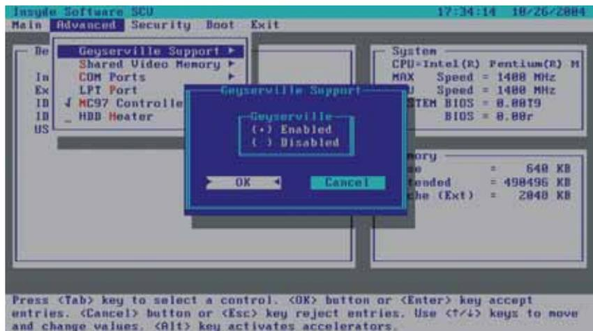
Allows maximum CPU performance when using AC/car power but minimum CPU performance when using battery power. The available options are *Enabled* and *Disabled*. Make sure that your CPU & OS supports this function.
