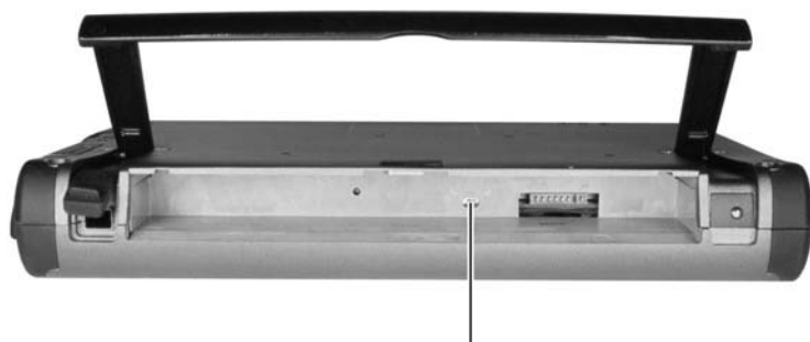
Backup Battery Switch
