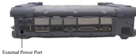
Figure 2-4 Connecting the External Power Adapter
