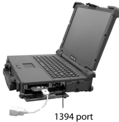
Figure 2-9 Removing IEEE 1394 Port
