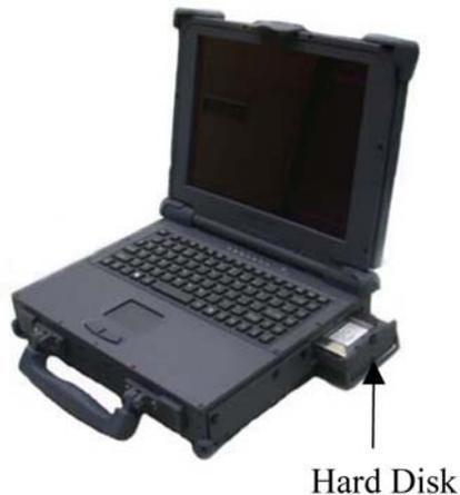
**Figure 2-8 Removing a Hard Disk Drive Module**
