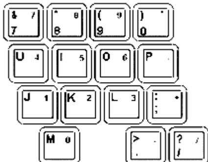
To activate the keypad, press the Num Lock key. The 15 keys shown in the figure switch from alphabetic keys to numeric keys. Press Num Lock again to return to alphabetic.
