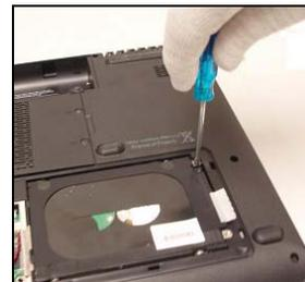
6. If there is a tab on the existing hard drive, gently pull it up and then to the outside to remove the hard drive from the bay.
