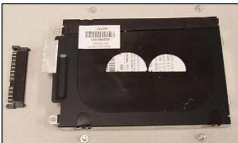
10. Align the SATA connector pins on the SSD with the SATA connector in the drive bay.
