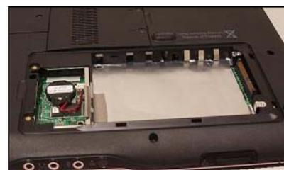
7. If your hard drive attaches to your motherboard via a cable, hold the cable's connector - not the cable itself - and gently remove the drive from it.
