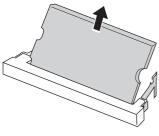
(2) Gently remove the RAM module from the slot.
