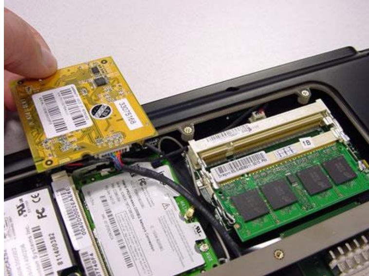
Fig. 5 Removing the Mini-PCI wireless card.
