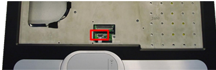
Fig. 11 Disconnecting touchpad flat cable
