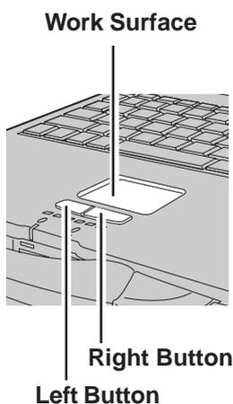
Use the touch pad to move the cursor on the display and perform normal computer operations. For instructions on how to handle the touch pad, refer to page 14.
