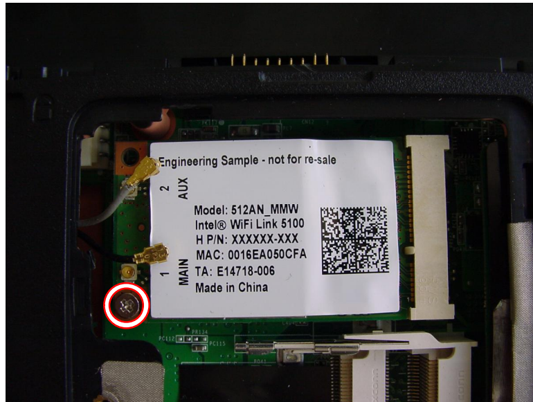
Fig. 13 Removing screw securing WLAN adapter.
