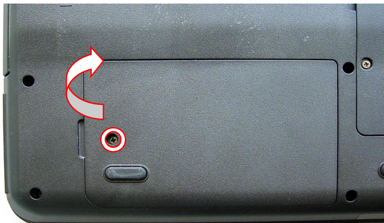
Fig. 2 Removing hard disk drive compartment cover.
