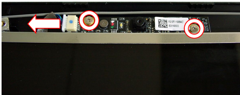
Fig. 41 Location of webcam connector.
