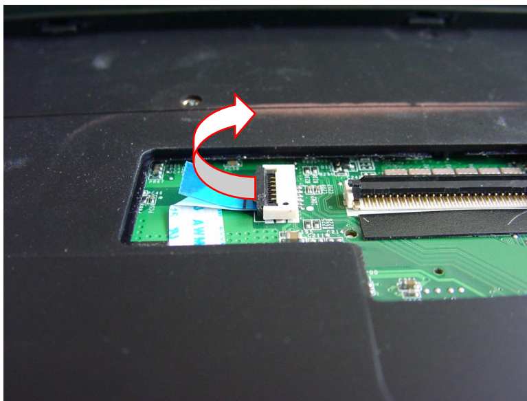
Fig. 23 Location of touchpad connector.
