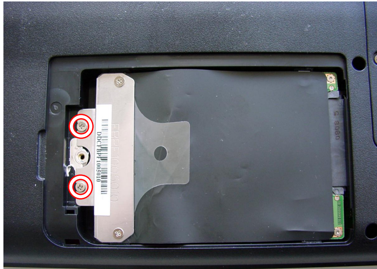
Fig. 3 Release hard disk drive.
