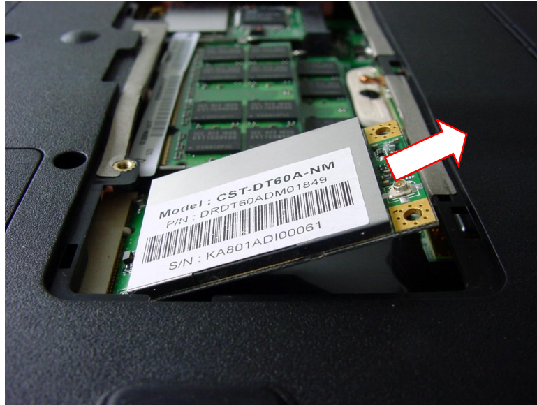
Fig. 17 Removing TV tuner card.
