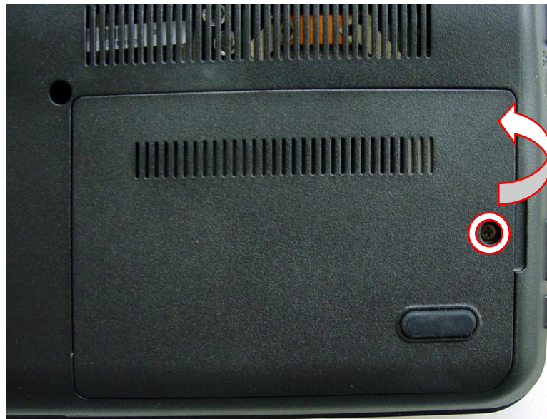
Fig. 6 Removing hard disk drive compartment cover.
