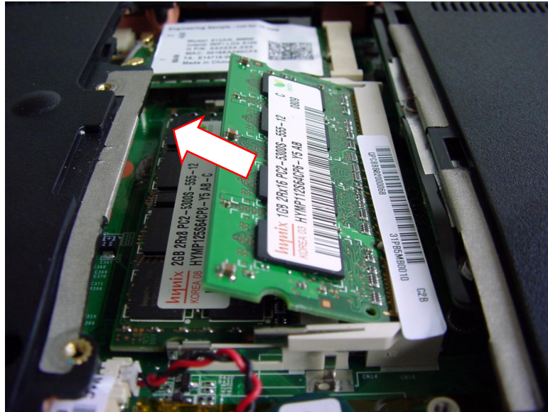
Fig. 11 Removing memory module.
