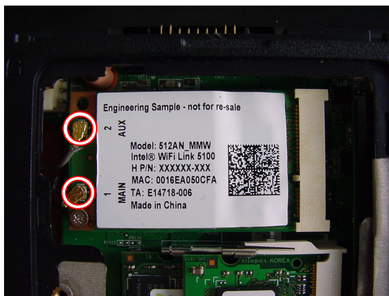
Fig. 12 Location of antenna cable connectors.
