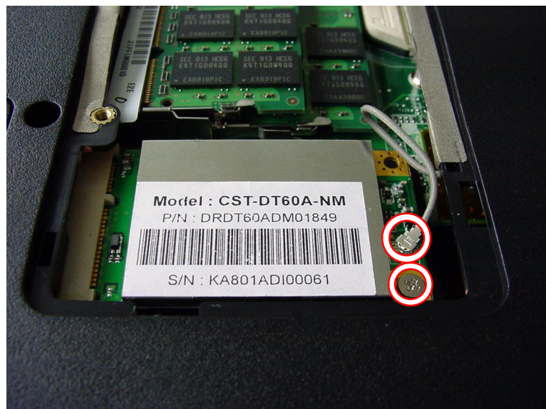
Fig. 16 Location of antenna cable connector and screw.
