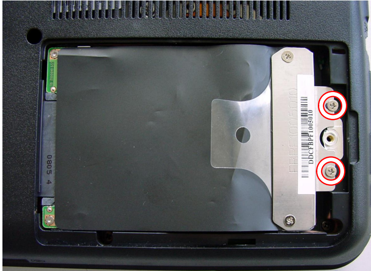
Fig. 7 Disconnecting and removing hard disk drive.
