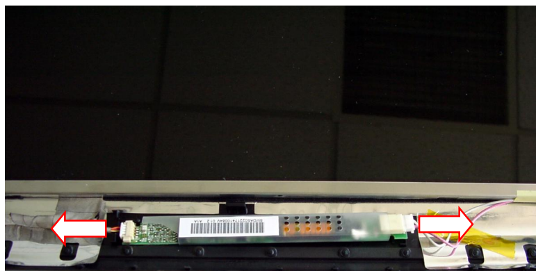
Fig. 40 Location of inverter board.
