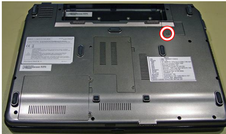
Fig. 14 Location of wireless LAN compartment cover screw.
