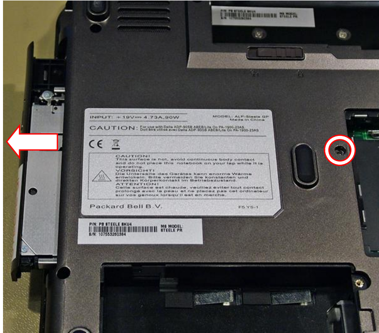
Fig. 7 Location screw securing optical disk drive.
