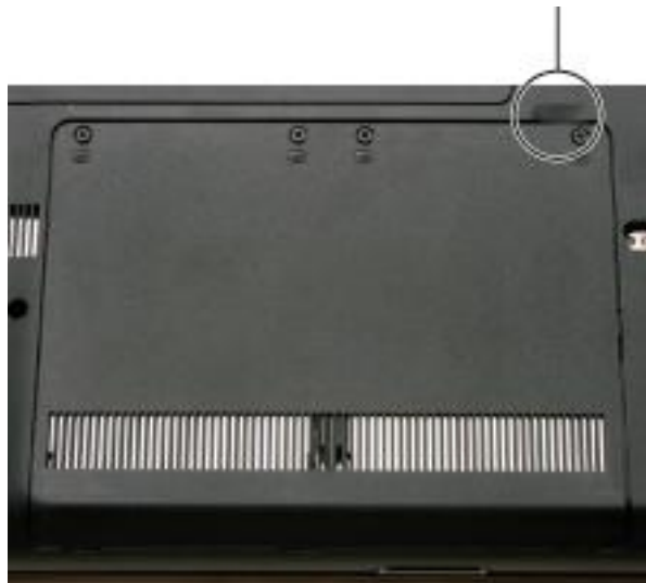
Fig. 16 Removing the hard disk drive bay cover.
