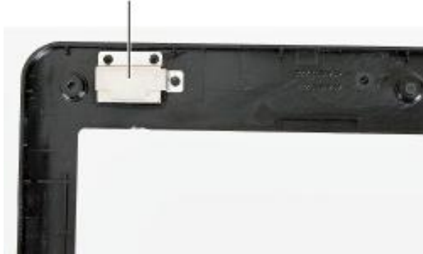
Fig. 49 Location of the LCD panel magnet bracket.
