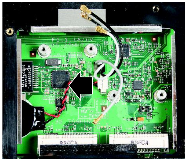
Fig. 14 Disconnecting the RTC battery.
