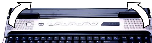
Fig. 25 Releasing the keyboard cover.
