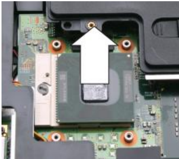
Fig. 10 Removing the CPU.
