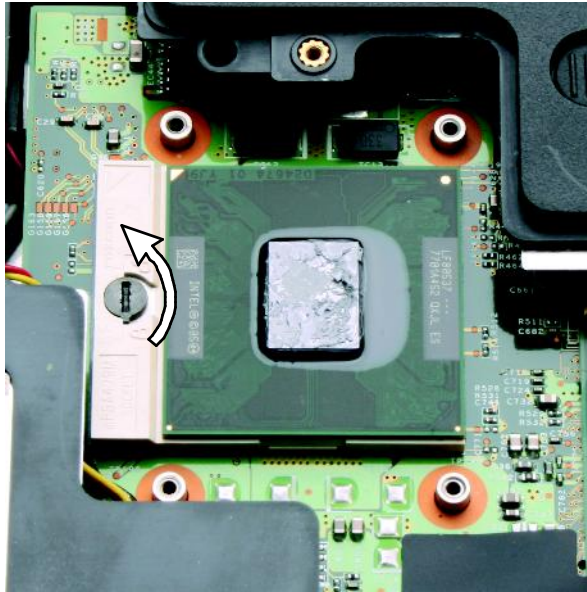
Fig. 9 Releasing the CPU screw.
