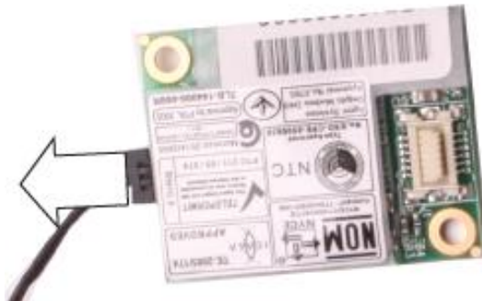
Fig. 65 Releasing the modem cable.
