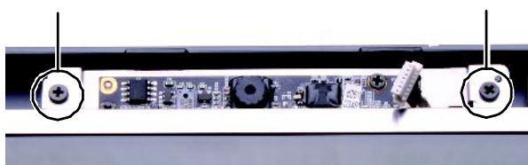
Fig. 41 Location of the webcam module screws.
