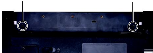
Fig. 23 Location of the keyboard cover screws.
