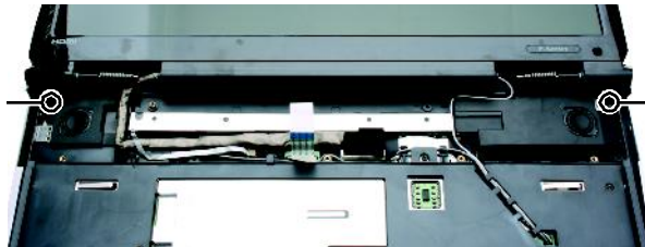
Fig. 46 Location of the LCD assembly hinge screws (top).
