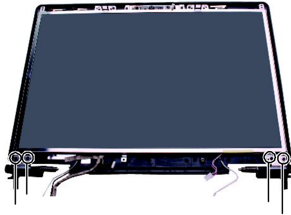
Fig. 48 Location of the LCD panel screws.
