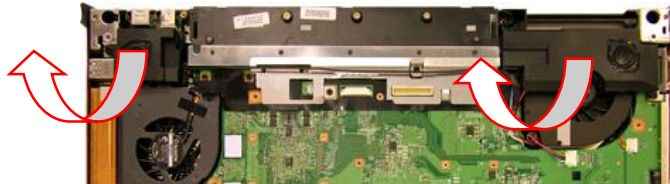
Fig. 68 Removing the speaker assembly.
