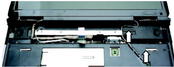
Fig. 45 Disconnecting the WLAN antenna cables.
