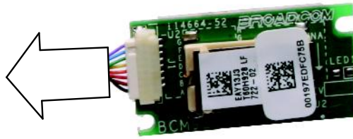
Fig. 62 Disconnecting the Bluetooth cable.
