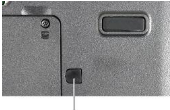
Fig. 20 Removing the DVD drive screw cover.
