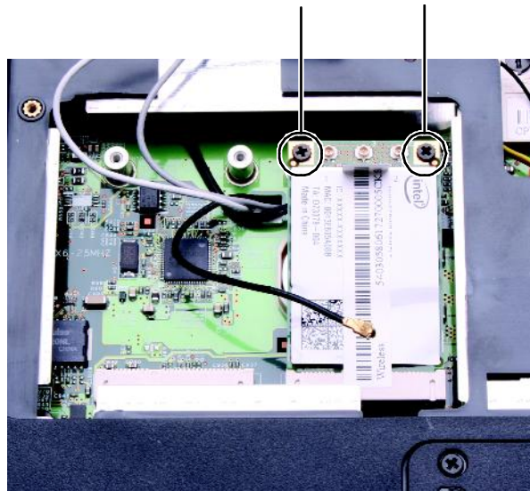
Fig. 12 Location of the wireless LAN adapter screw.
