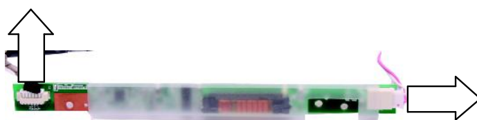
Fig. 39 Disconnecting the inverter cables.
