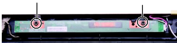
Fig. 37 Location of the inverter screws.
