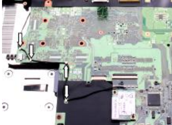
Fig. 70 Clearing the modem cables.
