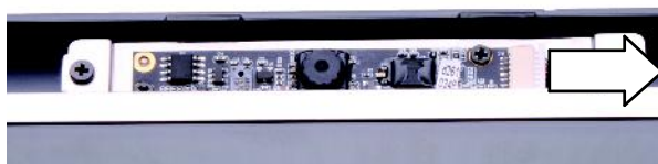
Fig. 40 Location of the webcam connector.
