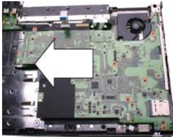
Fig. 74 Extracting the main board.
