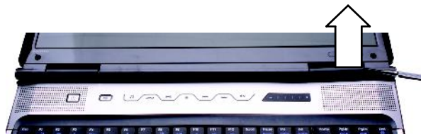
Fig. 24 Opening the hinge covers.
