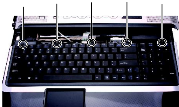
Fig. 32 Location of the keyboard screws.
