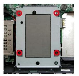
Fig. 27 Screws on the HDD holder
