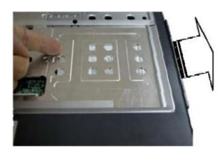
Fig. 10 Pushing the optical drive out
