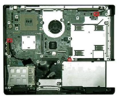
Fig. 28 Screws and connectors on Main Board
