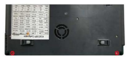
Fig. 12 Bottom screws retaining the LCD Module
