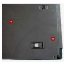
Fig. 9 Releasing the optical disk drive
