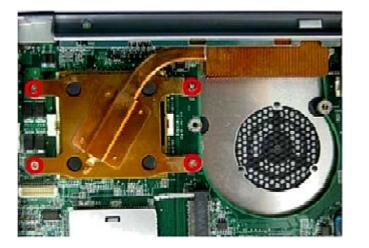
Fig. 20 Removing the CPU heat sink screws
