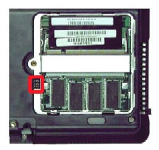
Fig. 32 Dip Switches location
