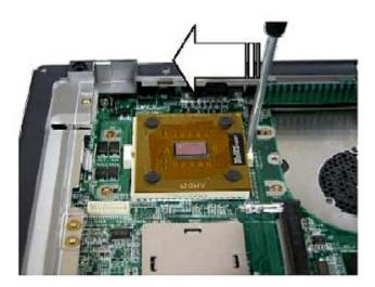
Fig. 21 Unlocking the CPU
