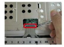
Fig. 8 Disconnecting the keyboard flat cable
