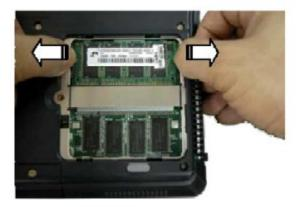
Fig. 3 Removing the memory module
