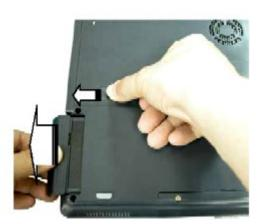
Fig. 1 Releasing the battery
