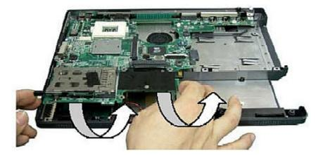
Fig. 29 Lifting up carefully the main board
