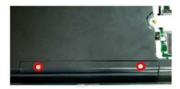
Fig. 4 Removing the hard disk drive cover
