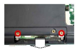
Fig. 5 Screws retaining the HDD assembly
