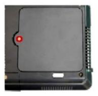
Fig. 2 Removing the screw retaining the memory cover
