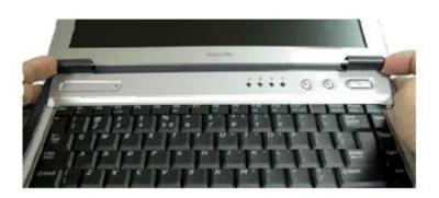
Fig. 7 Lifting up the keyboard cover
