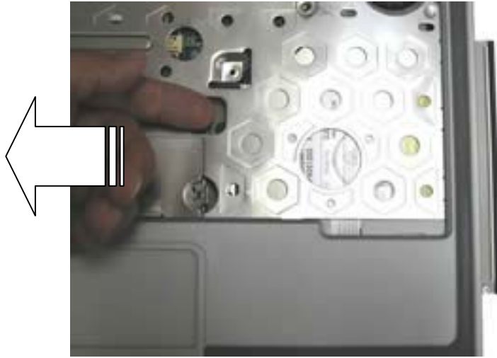
Fig. 12 Removing Heat plate from base unit
