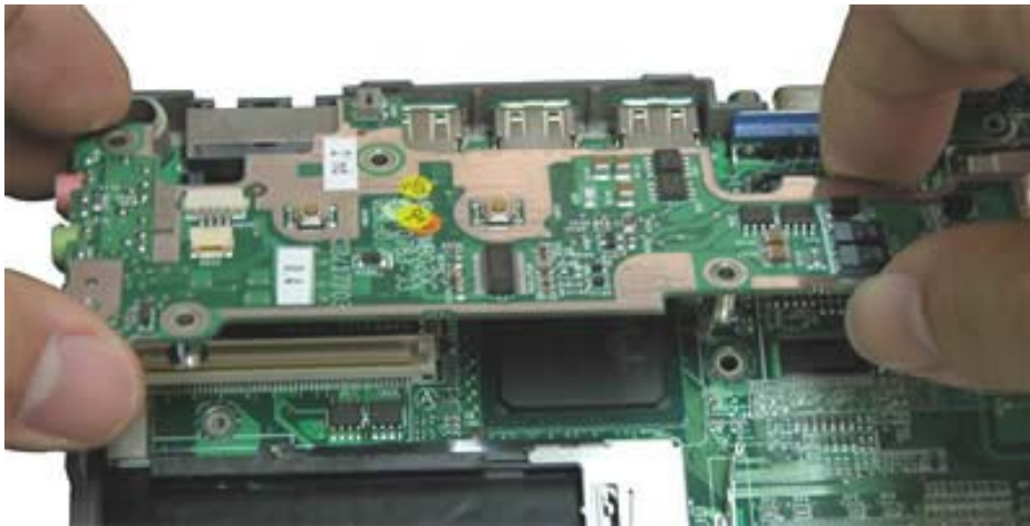
Fig. 32 Removing the DC/DC Board
