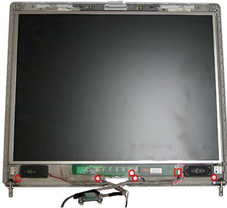
Fig. 24 Removing the inverter board screws
