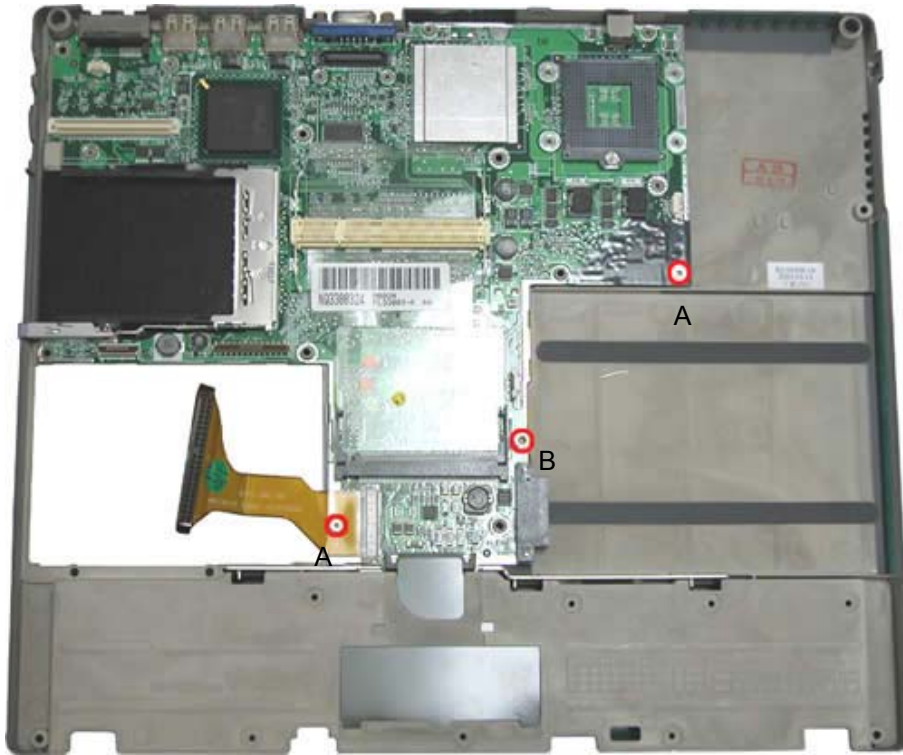
Fig. 33 Removing the main board screws
