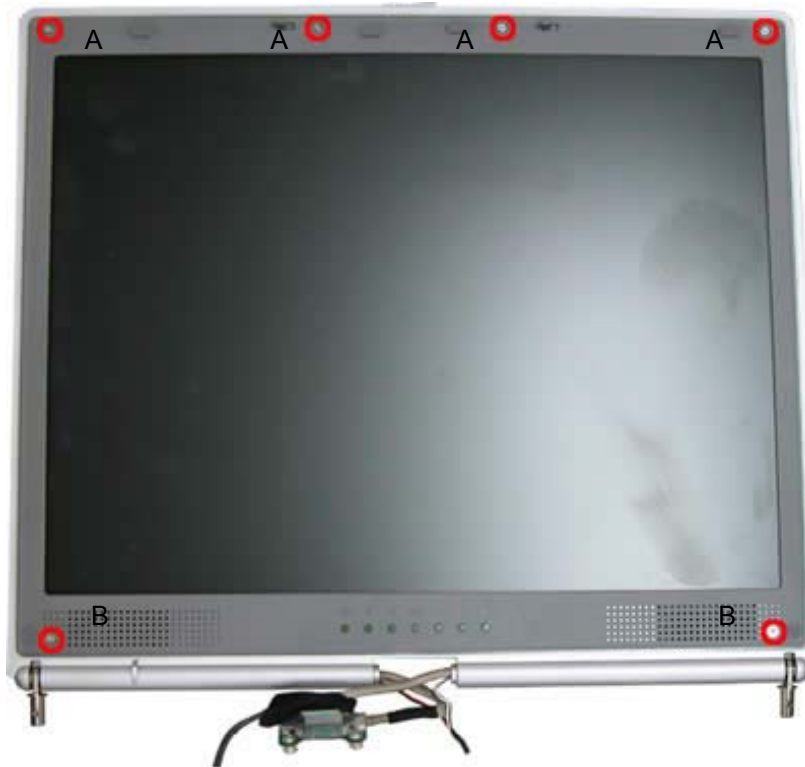
Fig. 22 Screws on the LCD Module
