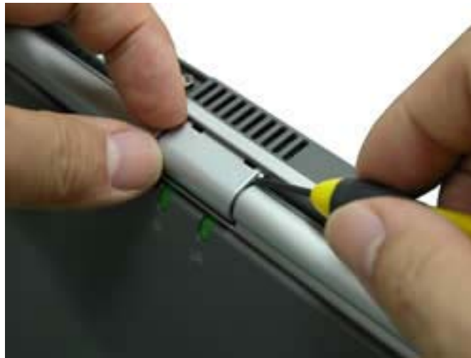
Fig. 19 Removing the LCD cable Cover
