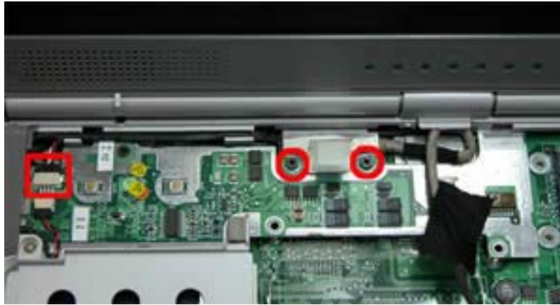
Fig. 18 Disconnecting the LCD & speaker connectors
