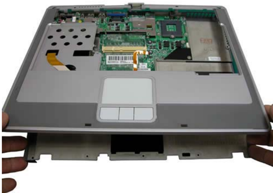
Fig. 29 Removing the top cover
