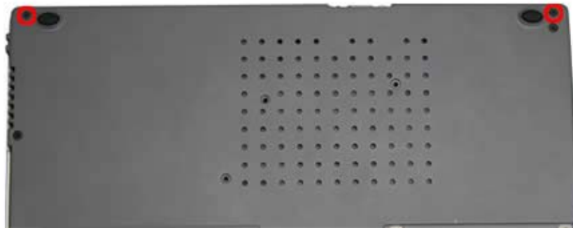
Fig. 21 LCD hinge screws at the bottom
