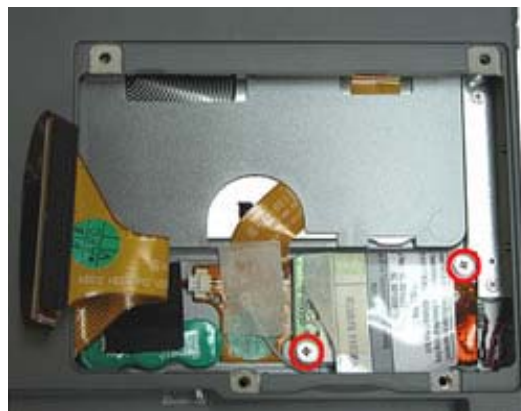
Fig. 5 Removing the screws on the MCD modem
