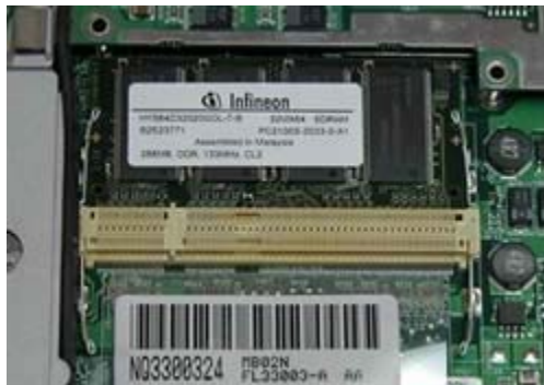
Fig. 13 Removing the memory module
