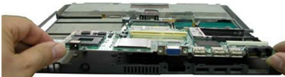
Fig. 35 Removing Main Board
