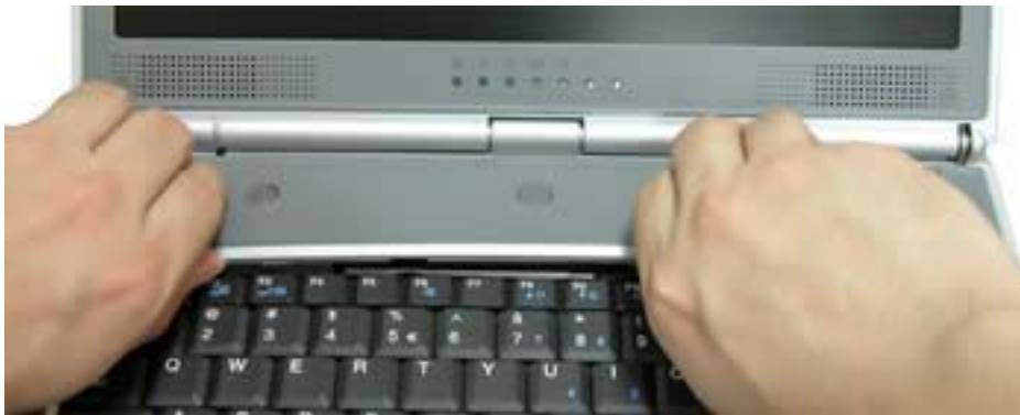
Fig. 7 Removing the Keyboard Cover
