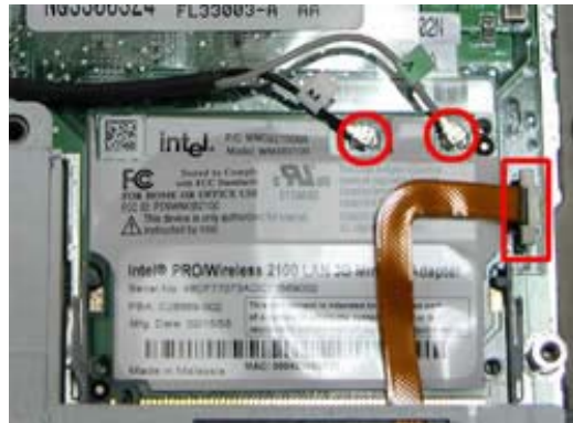
Fig. 14 Disconnecting the wireless antenna
