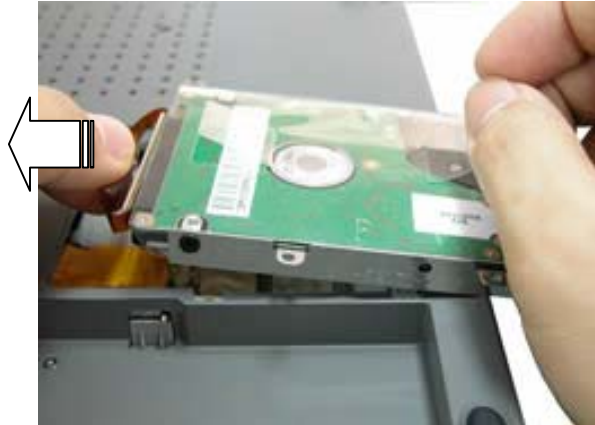
Fig. 3 Disconnecting the hard disk drive
