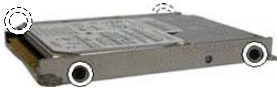
Fig. 4 Unscrewing the hard disk drive bracket screws
