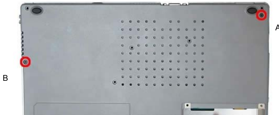
Fig. 27 Removing the Top cover screws on the bottom of the system
