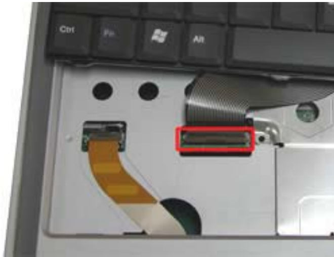
Fig. 9 Removing the keyboard FPC cable
