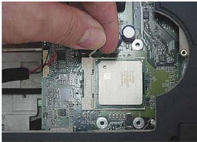
Fig. 31 Unlocking the CPU
