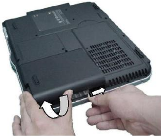
Fig. 1 Removing the battery
