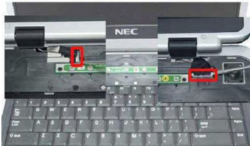
Fig. 13 Disconnecting LCD Connector
