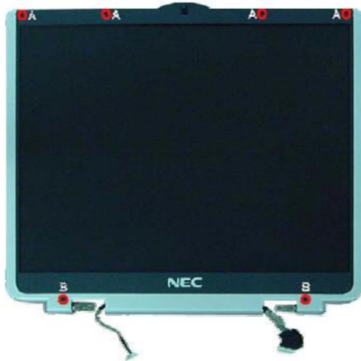
Fig. 17 Screws on the LCD Module
