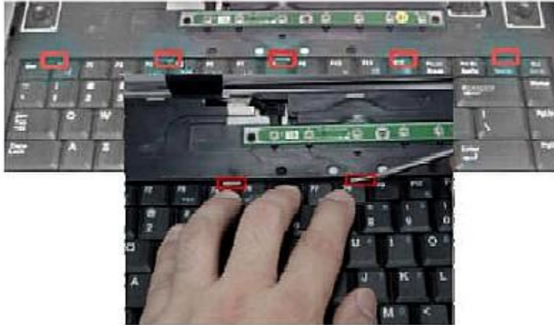
Fig. 9 Unlock the Keyboard
