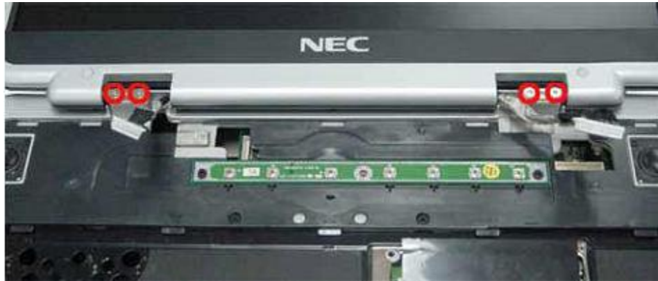
Fig. 15 Releasing the LCD Hinges
