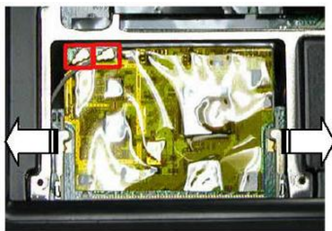
Fig. 41 Removing the WLAN Module
