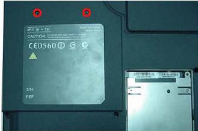
Fig. 5 Releasing the optical drive
