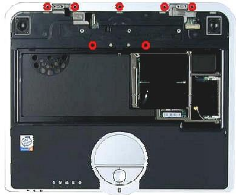
Fig. 33 Removing the top cover screws
