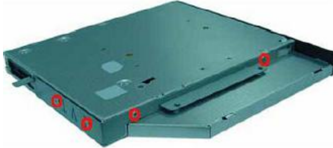
Fig. 7 Removing the Optical Drive Bracket
