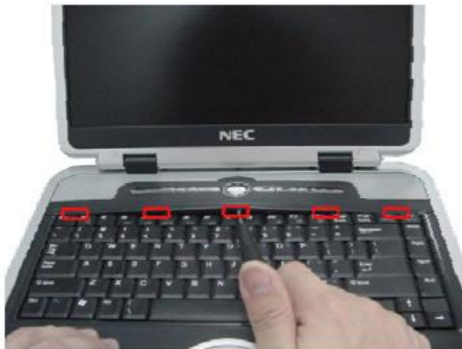
Fig. 8 Removing the Keyboard Cover
