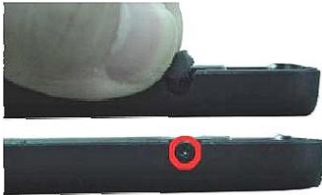
Fig. 20 Remove Side Rubber Covers
