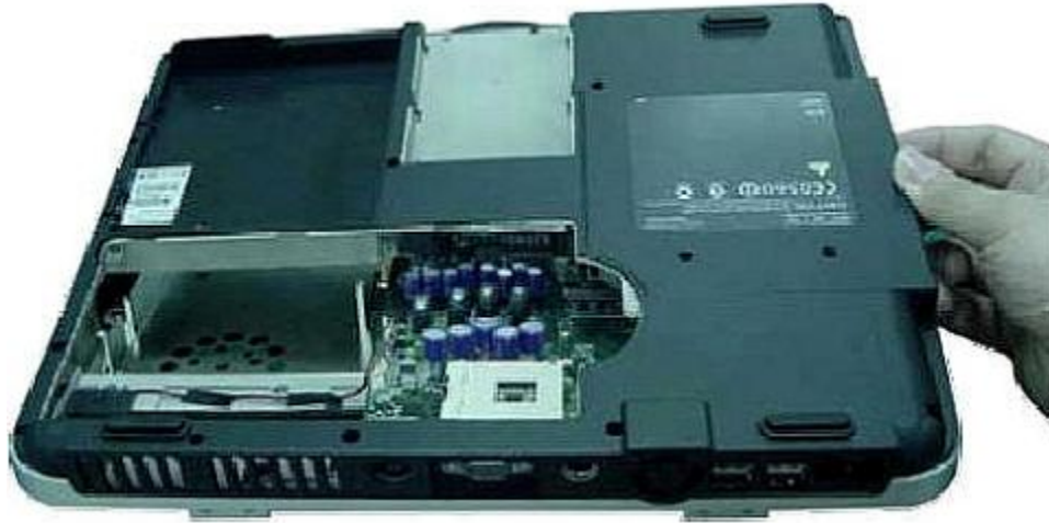
Fig. 36 Removing the Bottom Cover
