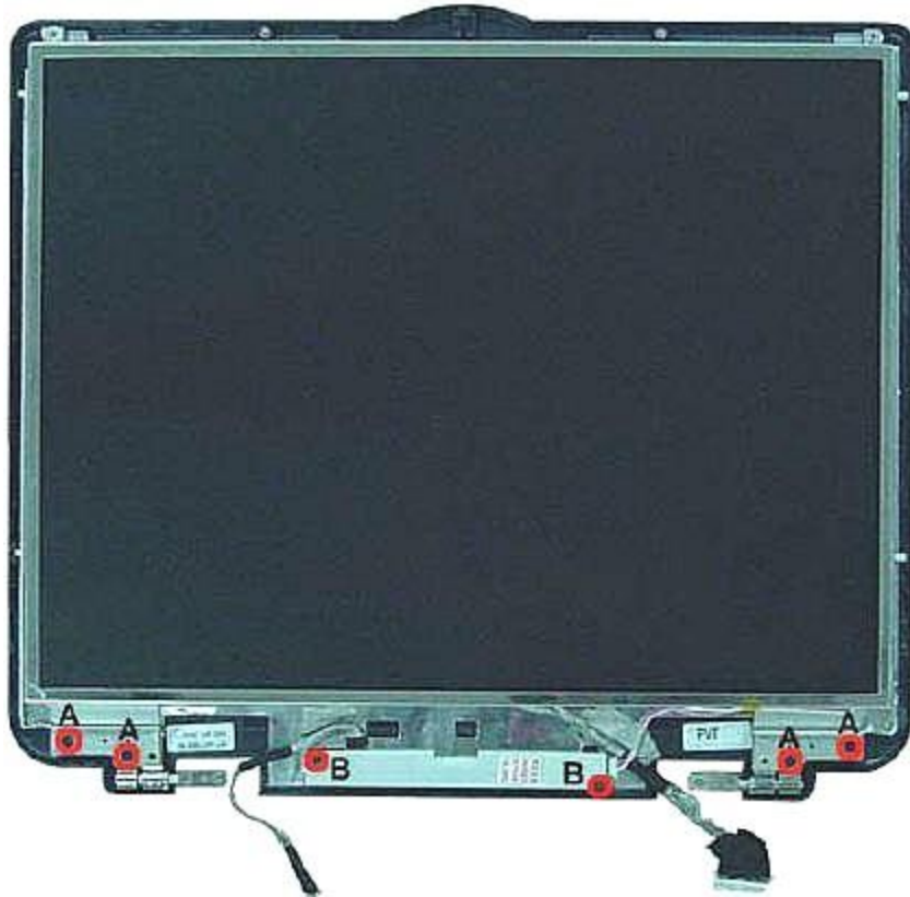
Fig. 19 Removing the LCD panel screws
