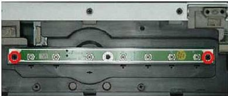
Fig. 32 Removing the Quick Key Board
