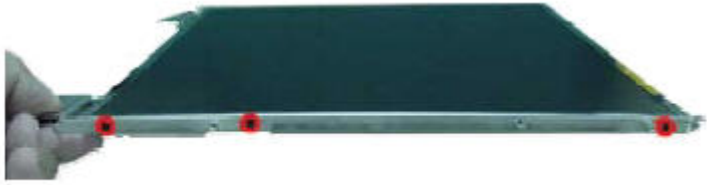
Fig. 27 Removing the LCD Panel hinges
