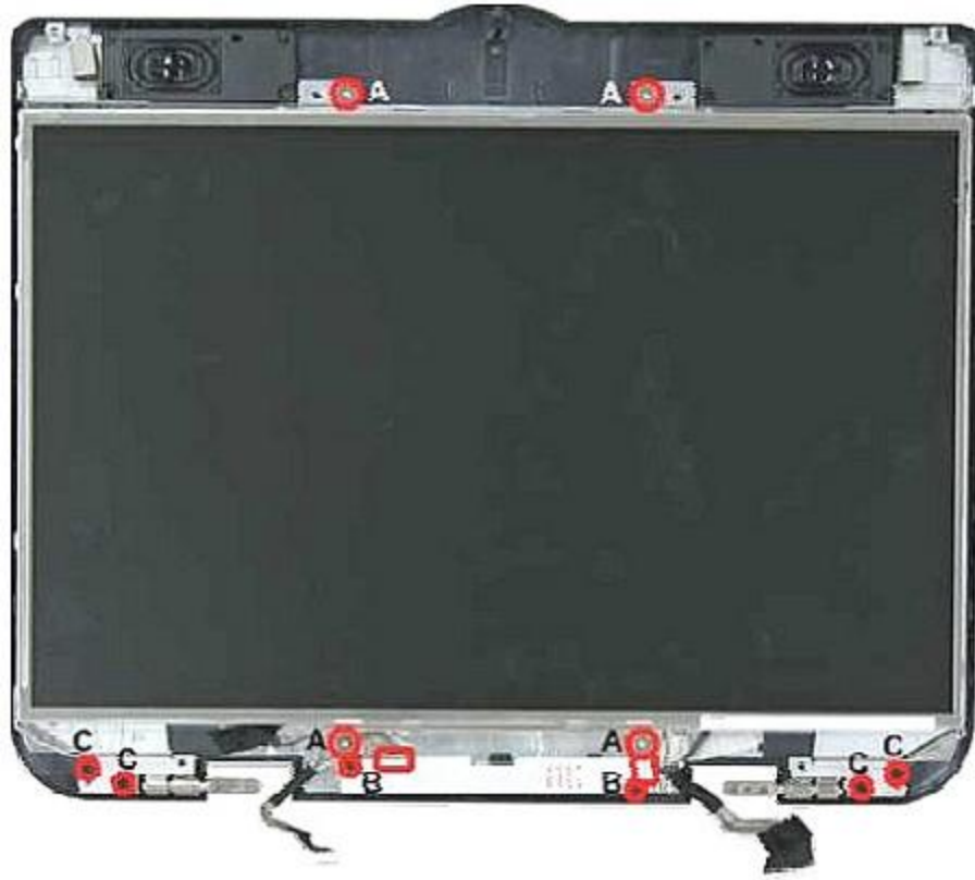
Fig. 25 Removing the LCD panel screws
