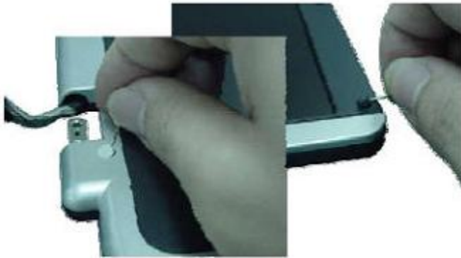
Fig. 22 Removing the rubber covers on the LCD Module
