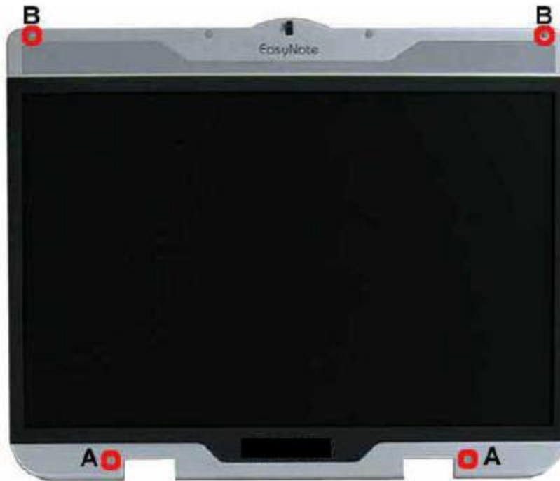
Fig. 23 Screws on the LCD Module
