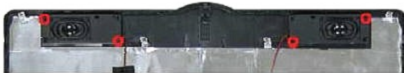
Fig. 28 Removing the Speakers
