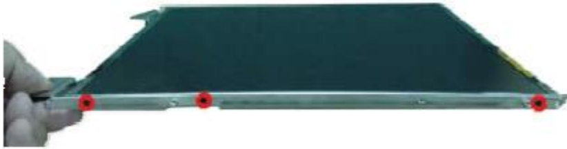
Fig. 21 Removing the LCD Panel hinges
