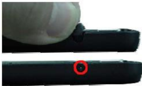
Fig. 26 Removing the side rubber covers
