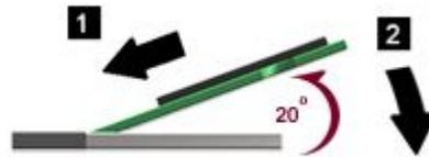
7. Pivot the SO-DIMM downward until it snaps into place.
