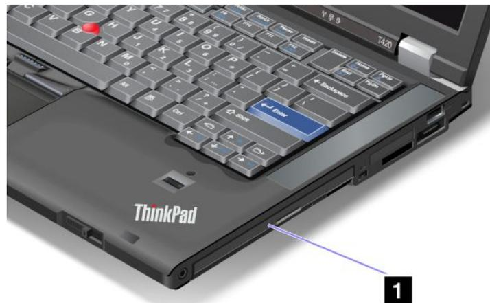
2. Insert the replaceable device into the bay; then press the device firmly into the connector.
