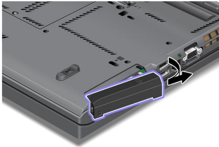
6. Remove the hard disk drive by pulling out the tab.
