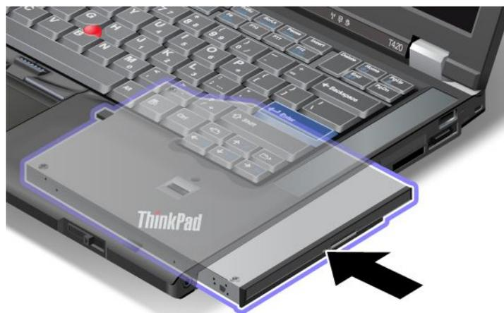
**Note:** If a hard disk password is set on a hard disk drive, you cannot hot-swap the drive. First remove the hard disk password, and then do the hot swap. Refer to “Hard disk passwords” on page 91.
