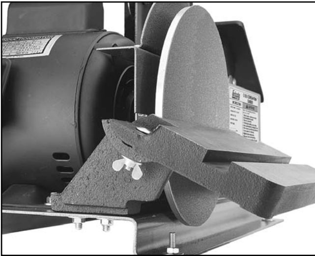
Figure 19. Disc table in tilted position.
