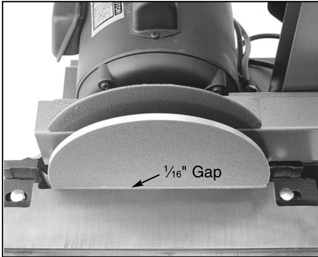
Figure 13. Table aligned with sanding disc.
