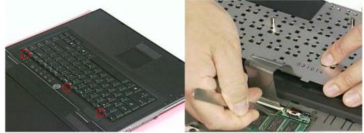
3. Remove 2 screws on the keyboard cover, then use tweezers to disconnect the keyboard two covers and lift it up.
