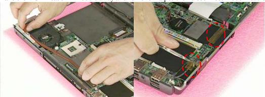
3. Loosen the audio FPC and FAN cable.
