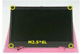
2. Prying the inside edges of the top front bezel, then separate it from LCD back cover and take LCD front bezel away.
