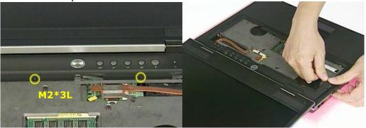
4. Loosen the switch board cable and take the keyboard cover away, then remove the switch cable
