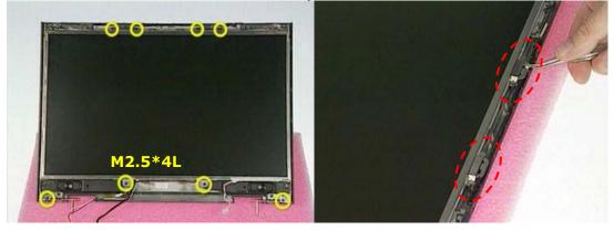
6. Remove 7 tapes \cdot 2 screws and 2 screws(M2\*3L(K)) on the other side.
