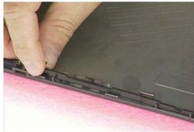
10. Remove 1 screw (M2.5\*4L(K)) and 1 screw on the other side, then take right and lift hinge off.
