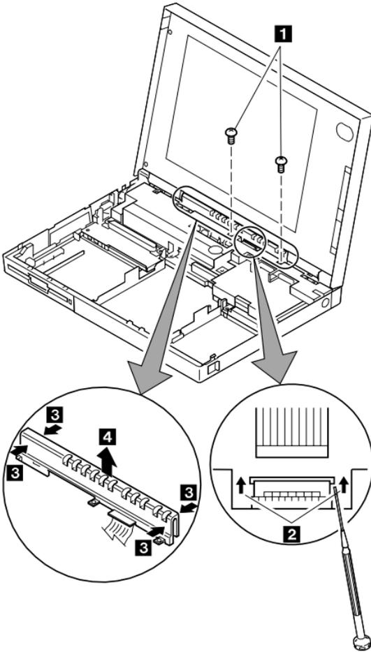
The status indicator has three latches on its rear and two in its front. In step **3**, do as follows:
