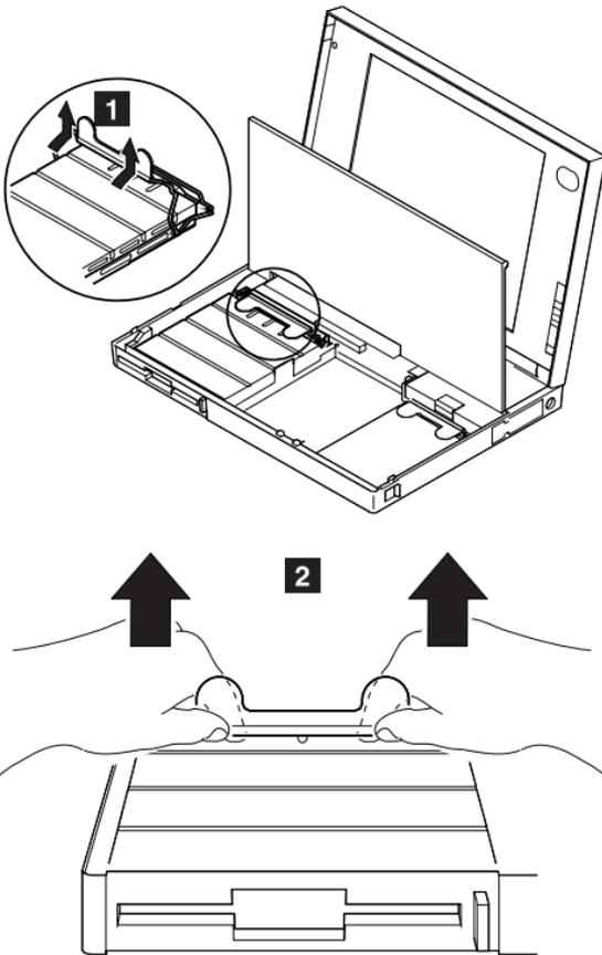
**Warning:** When replacing the diskette drive, check that the backup battery and standby battery are seated correctly to prevent damage to the diskette drive.
