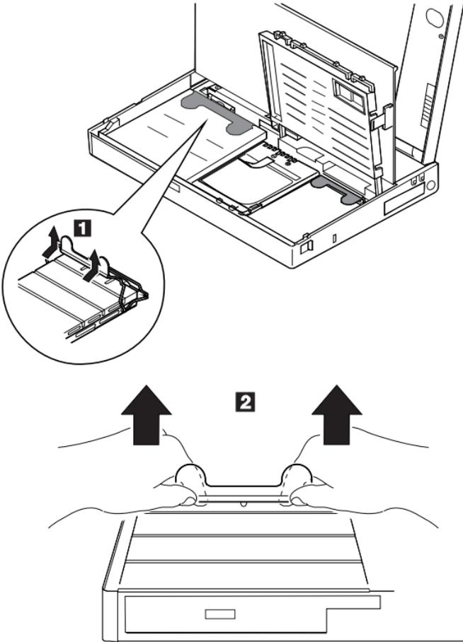
**Warning:** When replacing the CD-ROM/diskette drive, check that the standby battery is seated correctly to prevent damage to the drive.
