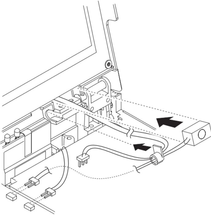
The right hinge should already be installed. To replace the microphone and cables, perform the following steps:
