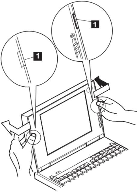
**Note:** While the cover is removed from the LCD, do not touch the film (**2**) on the rear cover.
