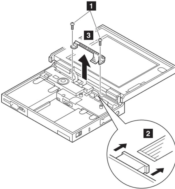
**Note:** When replacing the indicator, insert the flexible cable straight into the connector until the head of the cable stops. Slide both ends of the latches at the same time to make sure that the cable is correctly inserted.
