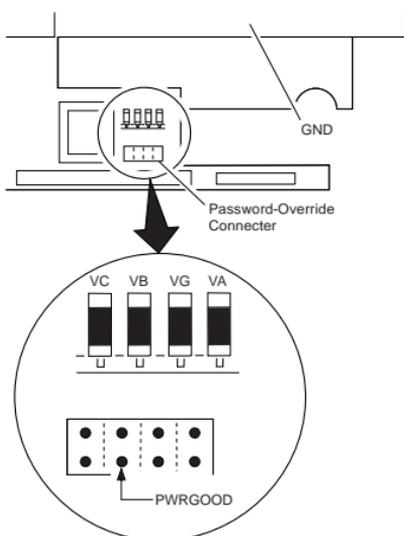
**Note:** Only VOLT is marked on the system board. Use the above figure to locate the VA, VG, VB, VC, and PWRGOOD signal names.
