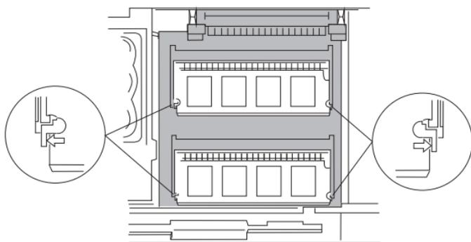
While holding the strap **1**, pull the DIMM adapter toward the front **2** to remove it.
