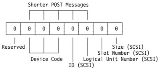
All SCSI devices are set to a different SCSI ID. Duplicate SCSI ID settings can generate a false error message. Use the SCSI ID to determine whether the error message is coming from an internal or an external device.
