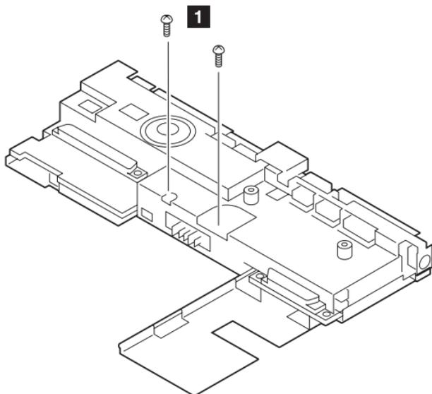
Turn the system board upside down. Then remove any metal tape holding the card.
