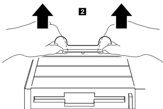
After replacing the diskette drive, latch the removal strap into the correct position.
