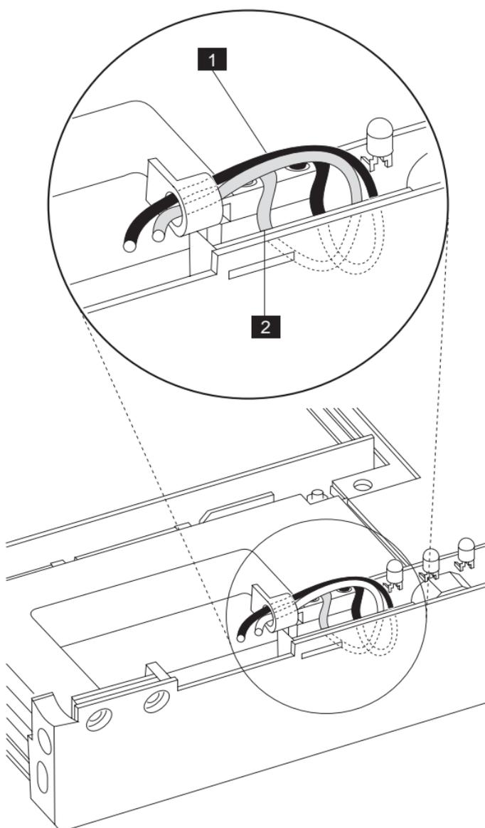
**Backlight cable routing from the rear, shown without the computer lid.**
