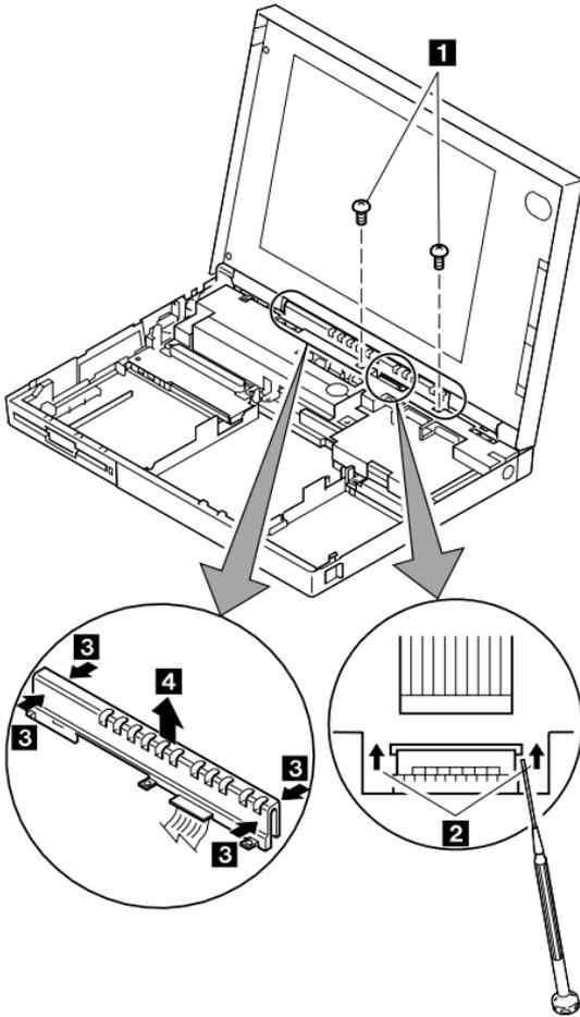
The status indicator has three latches on its rear side and one on its front side. For step **3**, do the following:
