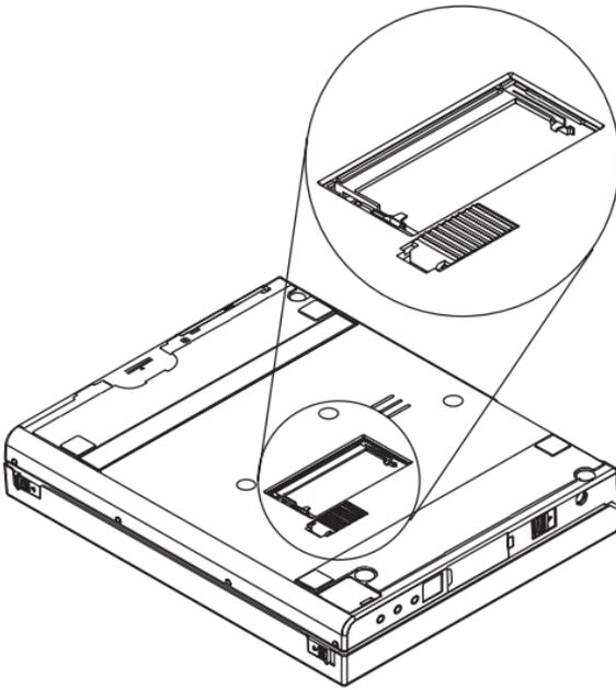
6. Press the metal tabs on each side of the SO-DIMM away from the card. The card should raise slightly as the tabs are pulled away from it.
