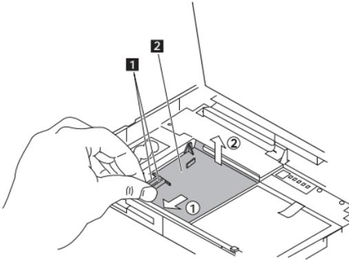
2. When inserting the DIMM into either connector on the DIMM adapter:
