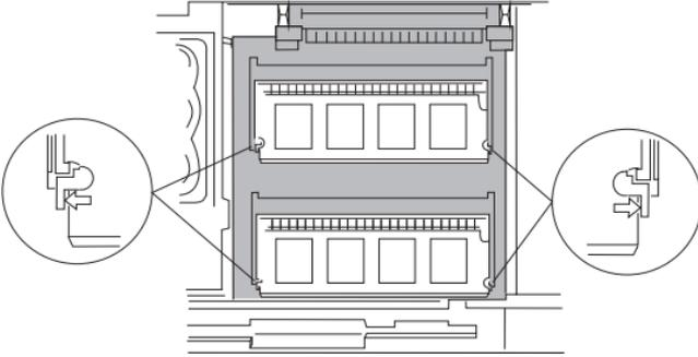
While holding the strap **A**, pull the DIMM adapter toward the front to remove it.
