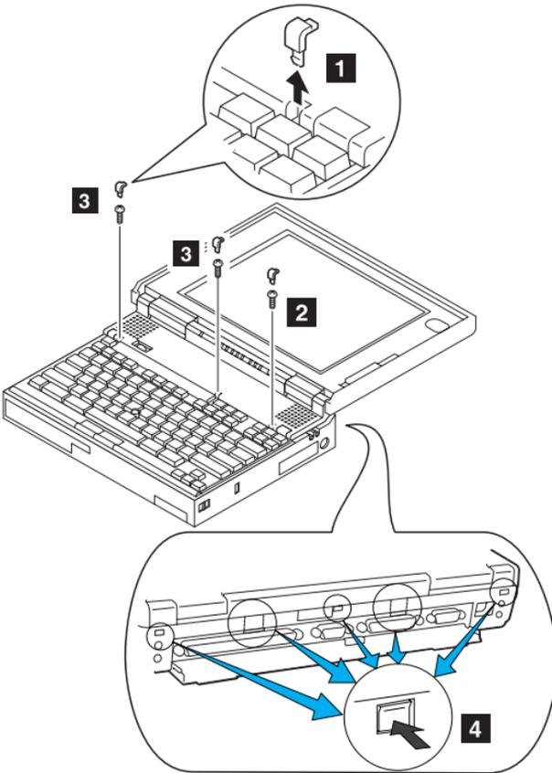
The keyboard unit is connected to the system board with flexible cables. Remove the upper cover; then disconnect the cables to remove the keyboard unit as shown.
