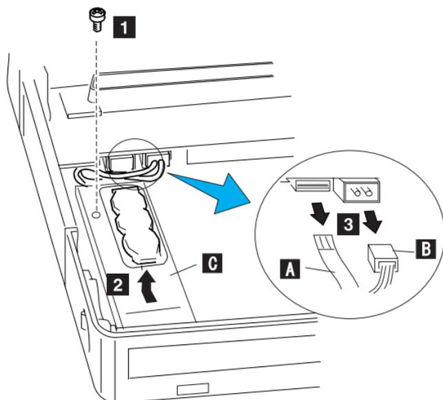
Where: **A** is the IR Cable. **B** is the Standby Battery Cable. **C** is the IR Lens.
