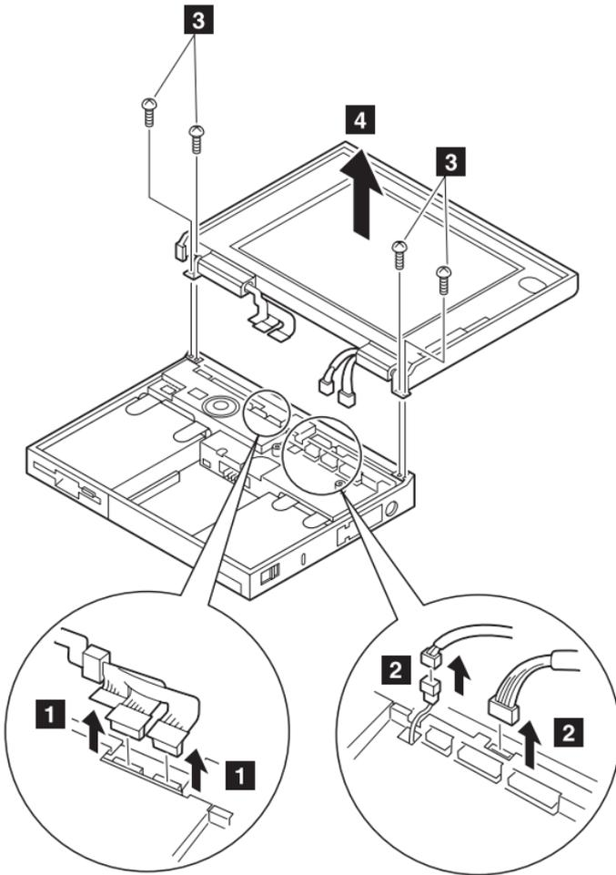
**Note:** When removing the LCD cables **1**, pull the connector straight up. Incorrect handling can damage the connector.
