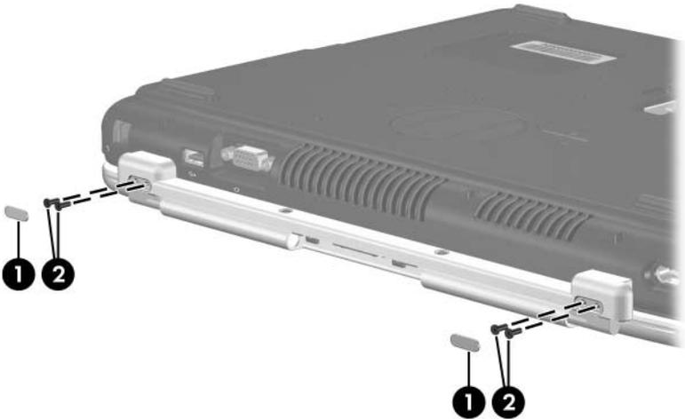
*Removing the Display Screws, HP Pavilion zv6000 Models*
