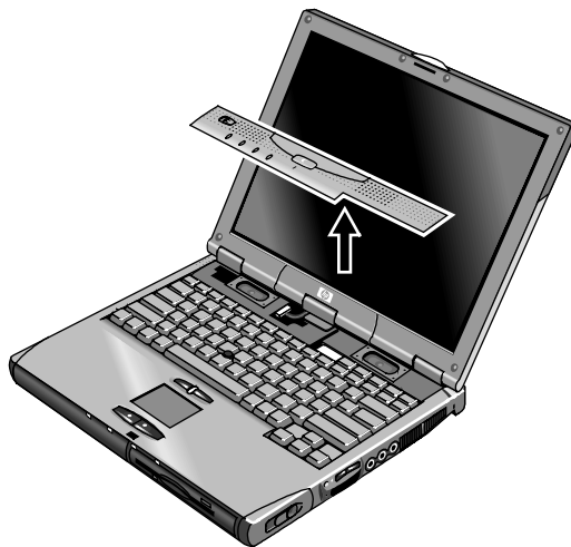
Figure 2-9. Removing the Power Button Panel
