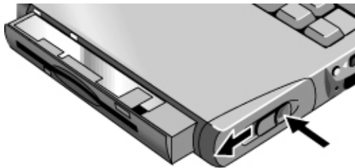
Figure 2-3. Removing a Module
