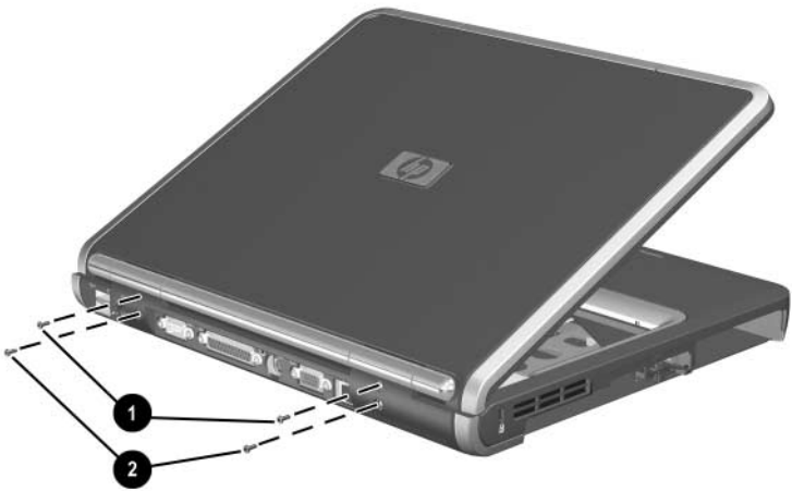
Removing the Display Screws
