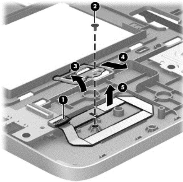
Reverse this procedure to install the fingerprint reader board.
