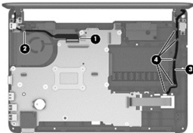
7. Remove the 2 Phillips PM2.0x4.0 screws (**1**) that secure the power connector bracket to the computer.
