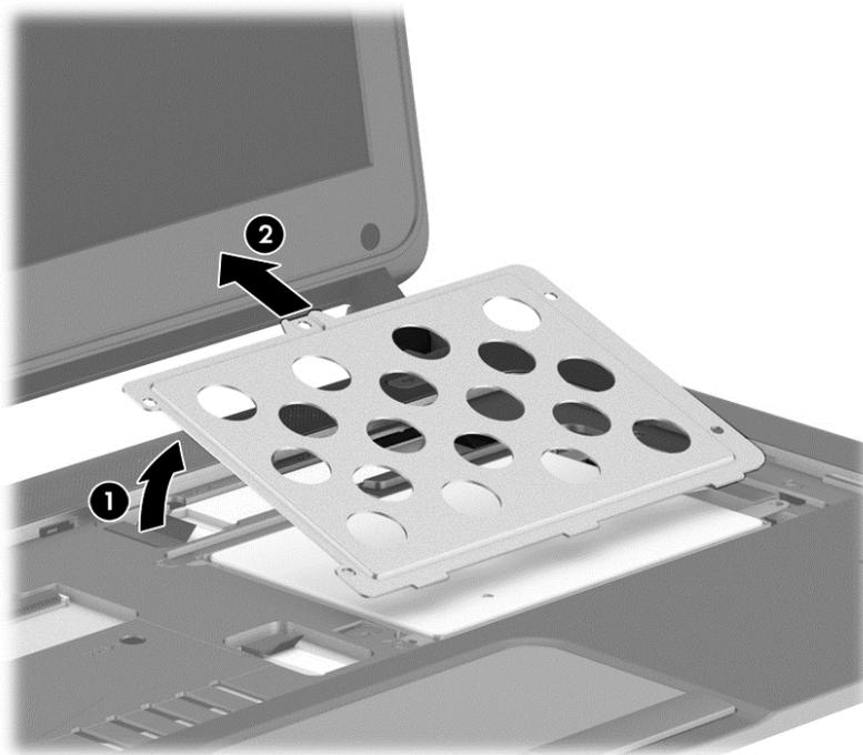
4. Pull the hard drive tab **(1)** toward the edge of the computer to disconnect the hard drive.
