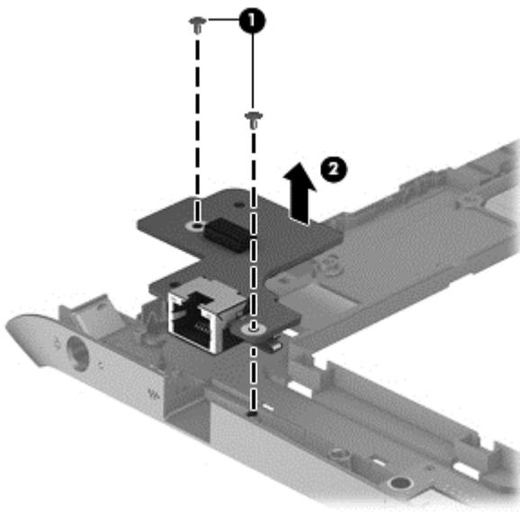
Reverse this procedure to install the function board.
