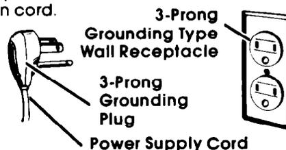
**DO NOT, UNDER ANY CIRCUMSTANCES, REMOVE THE POWER SUPPLY CORD GROUND PRONG.**
