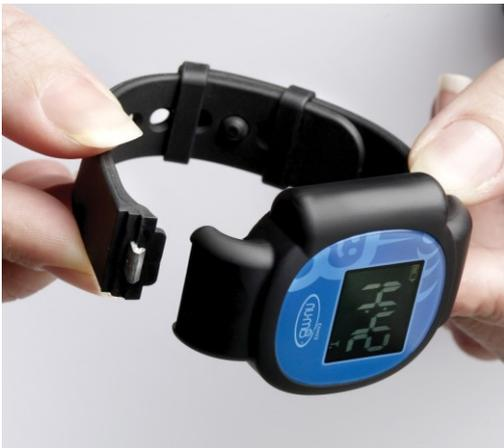
If the clock does not appear nu-m8 is not connected to the network. The most common reason for this is poor mobile phone coverage. If you take your child outside this will help it to acquire the necessary signal strength. Once coverage is established nu-m8 will hold the signal even in areas where it couldn't get signal at boot-up.
